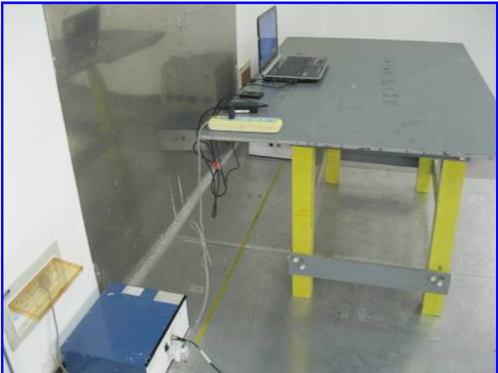
Conducted Emission Test Setup Side View
