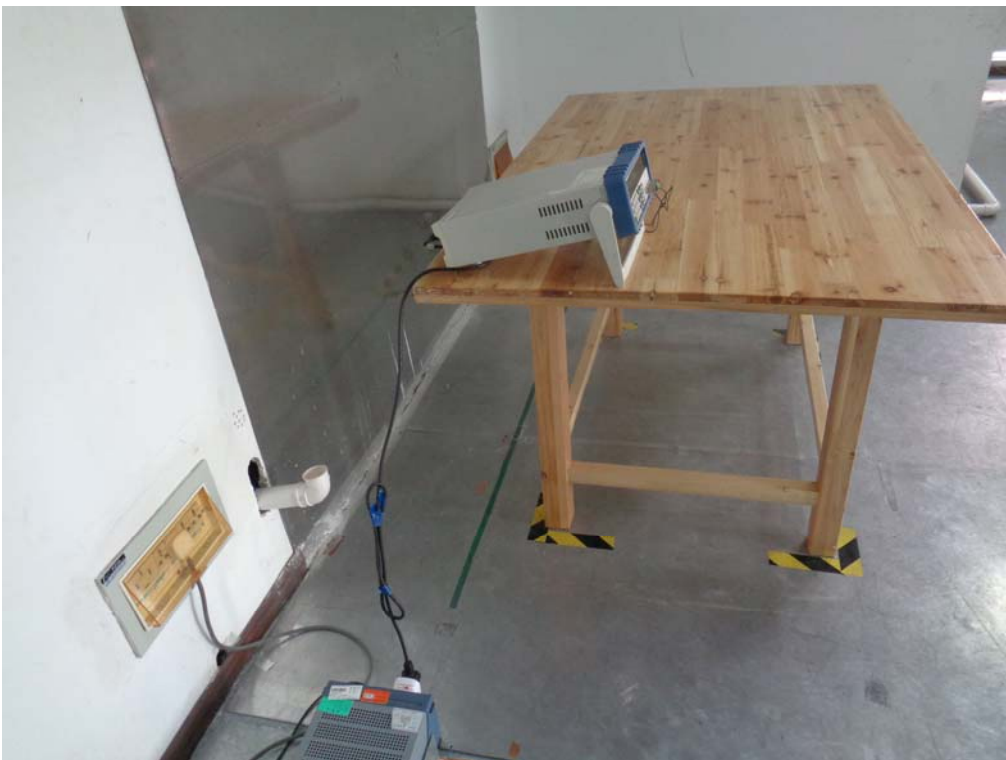
Conducted Emissions Setup Side View
