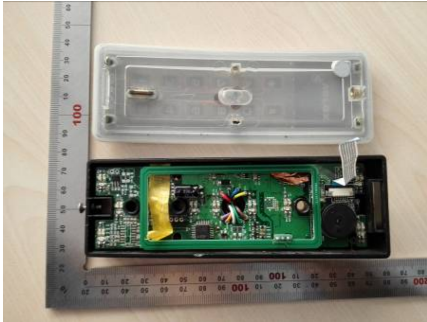
EUT – Main Board Top & Loop Antenna View
