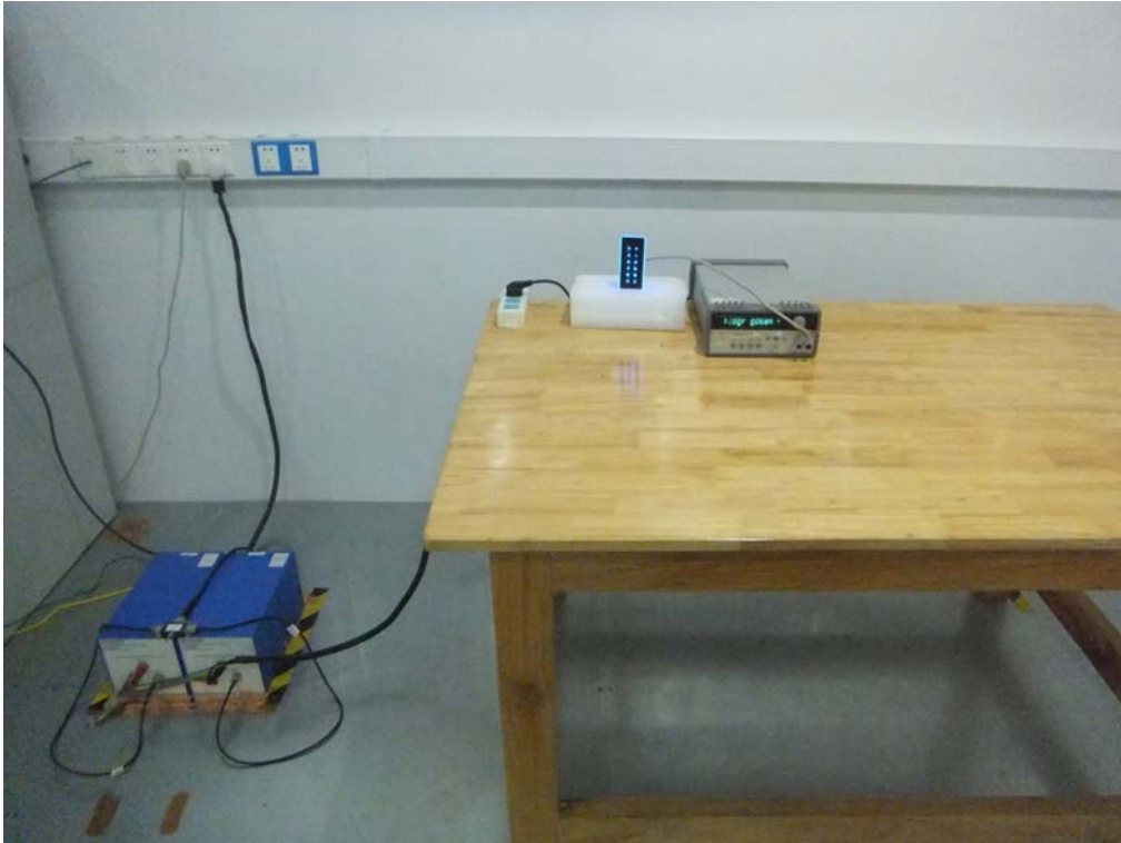
Conducted Emissions Setup Front View
