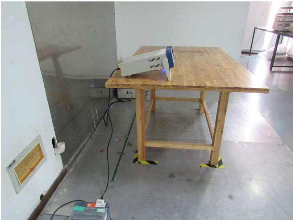
Conducted Emissions Setup Side View
