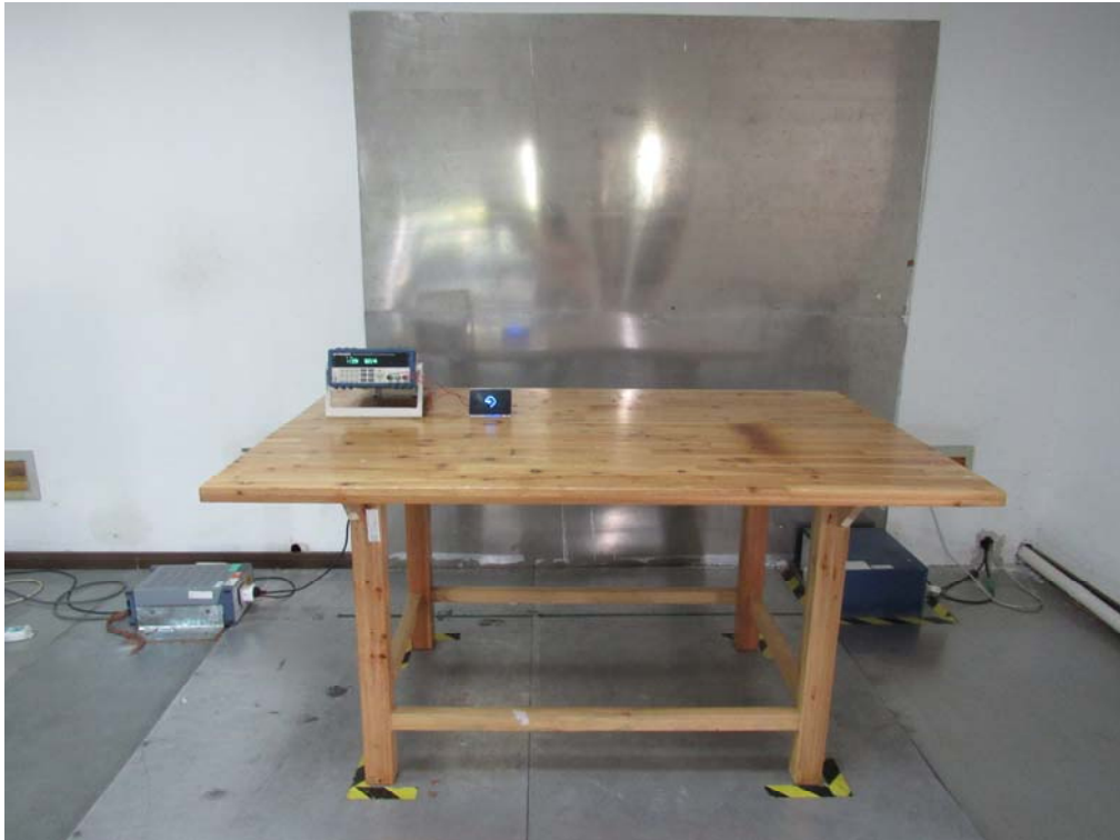
Conducted Emissions Setup Front View
