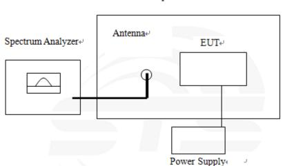
The EUT which is powered by the Battery, is coupled to the Spectrum Analyzer; the RF load attached to the EUT antenna terminal is 500hm; the path loss as the factor is calibrated to correct
