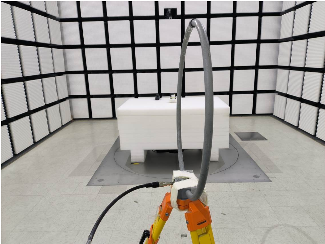
Radiated Emission 9k-30MHz Perpendicular View MW-322
