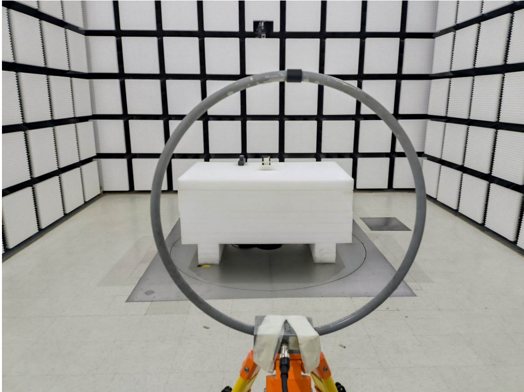
Radiated Emission 9k-30MHz Perpendicular View MW-322
