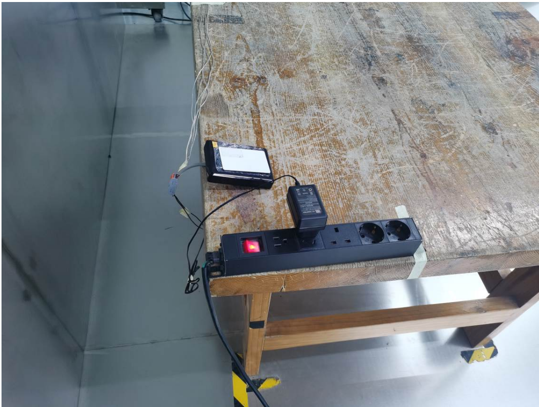
Conducted Emissions Side View MW-322
