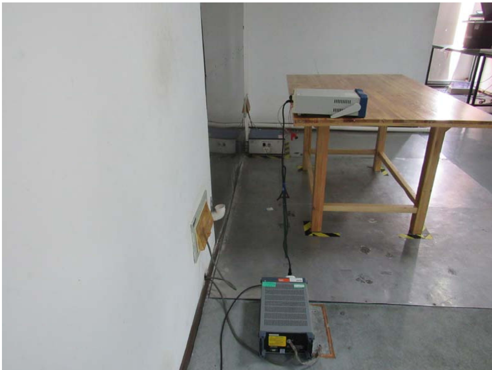
Conducted Emissions Setup Side View
