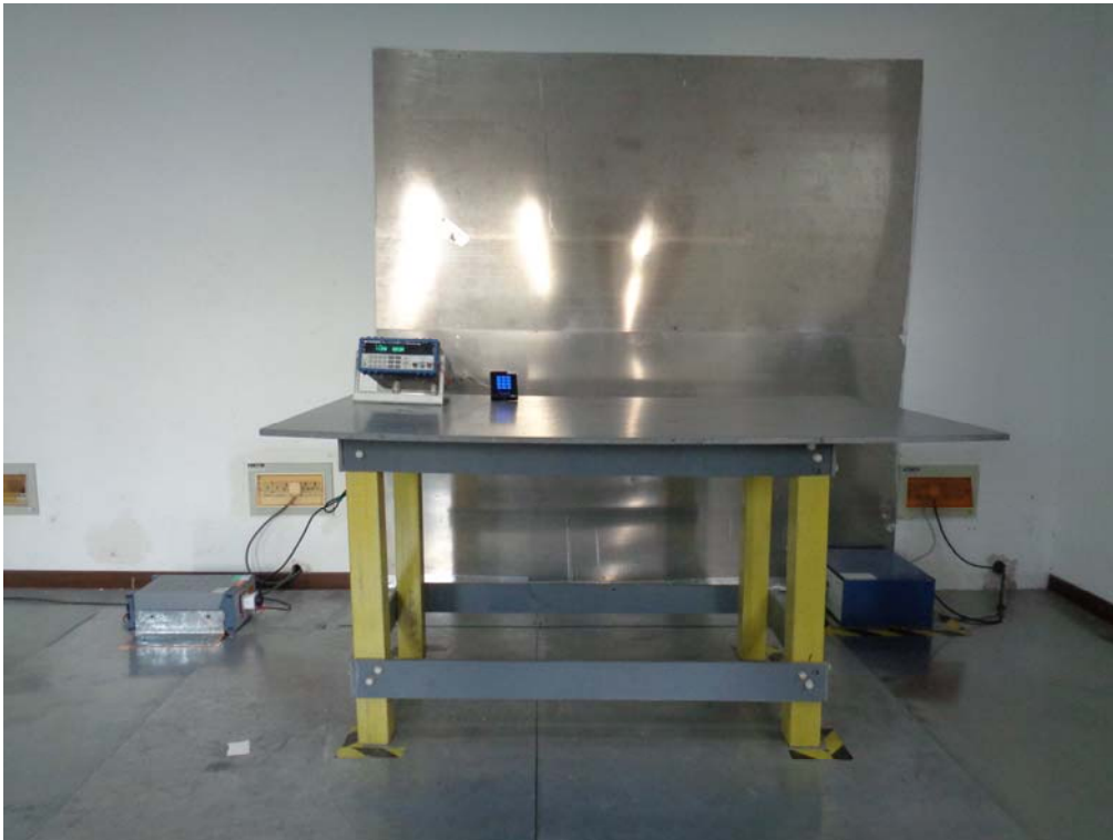
Conducted Emissions Setup Front View
