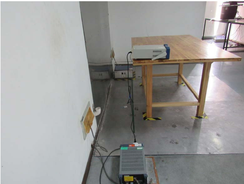
Conducted Emissions Setup Side View
