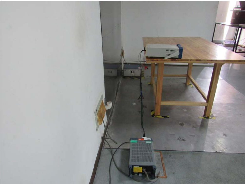
Conducted Emissions Setup Side View
