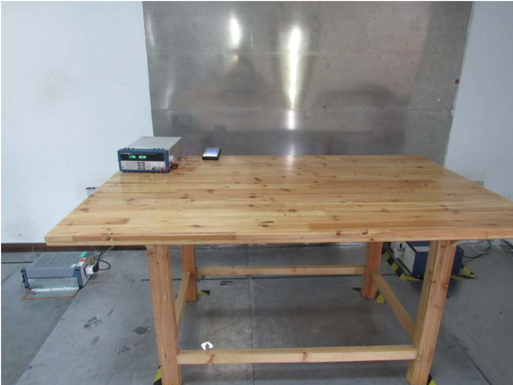
Conducted Emissions Setup Front View
