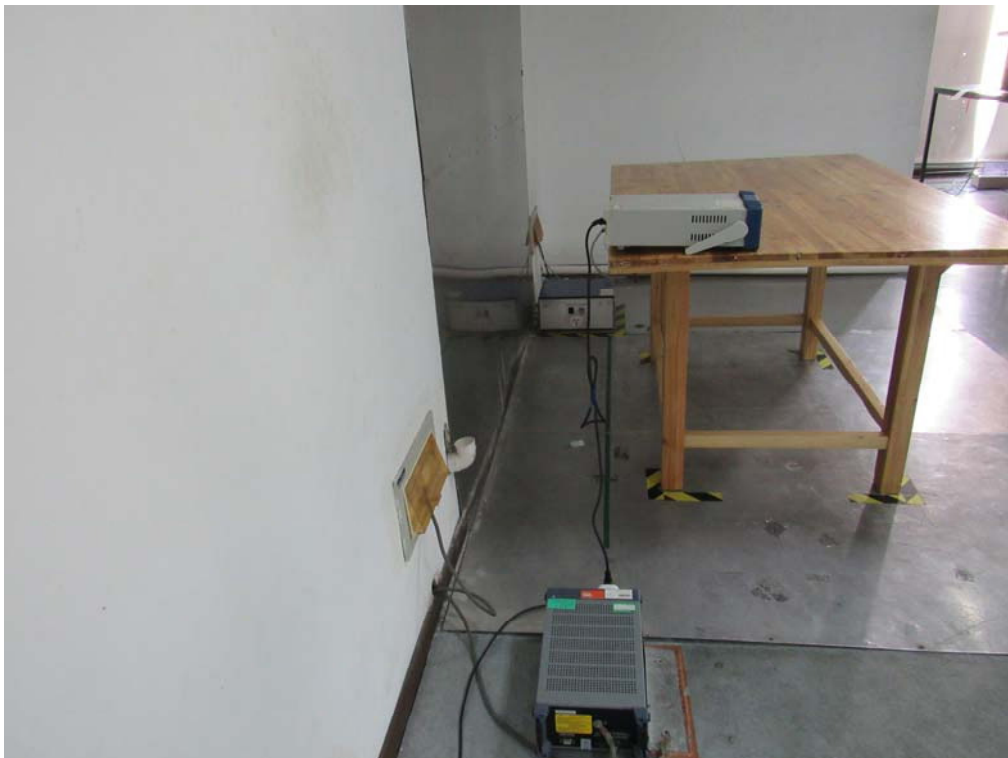
Conducted Emissions Setup Side View
