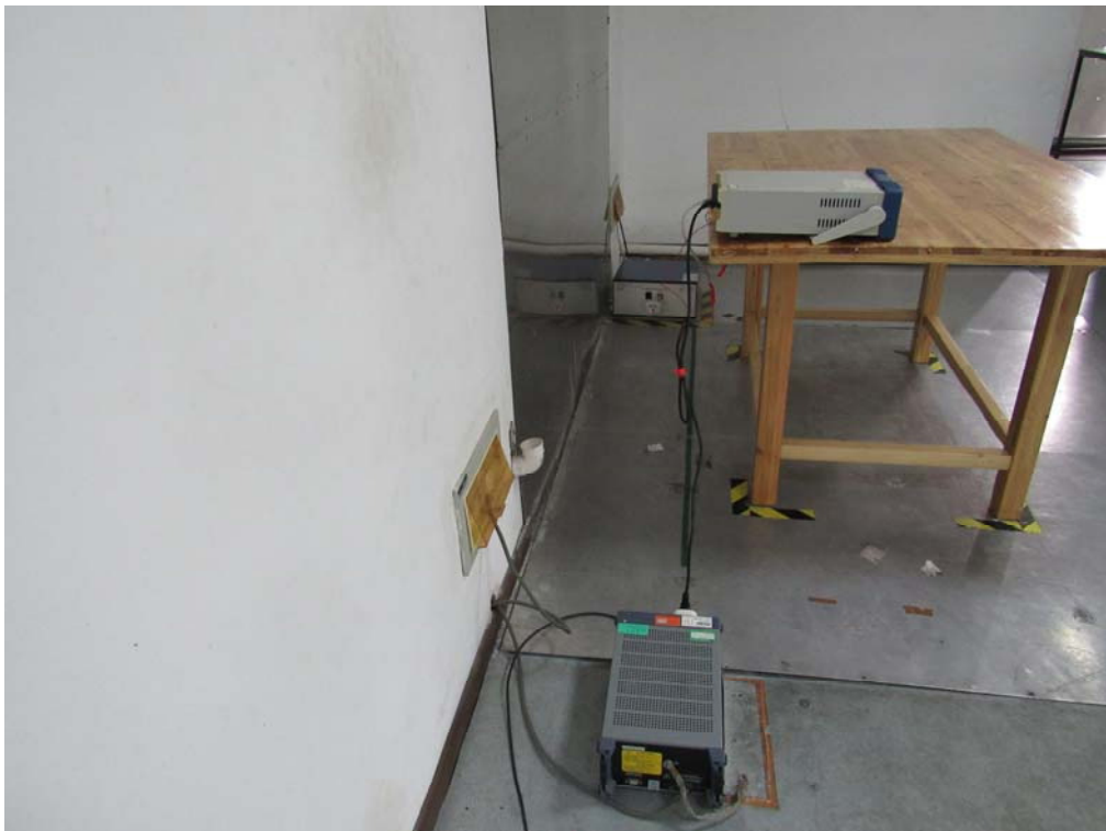
Conducted Emissions Setup Side View
