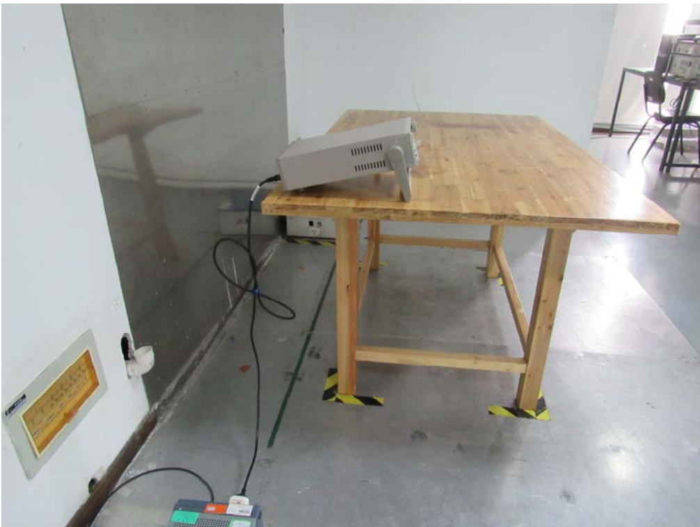
Conducted Emissions Setup Side View
