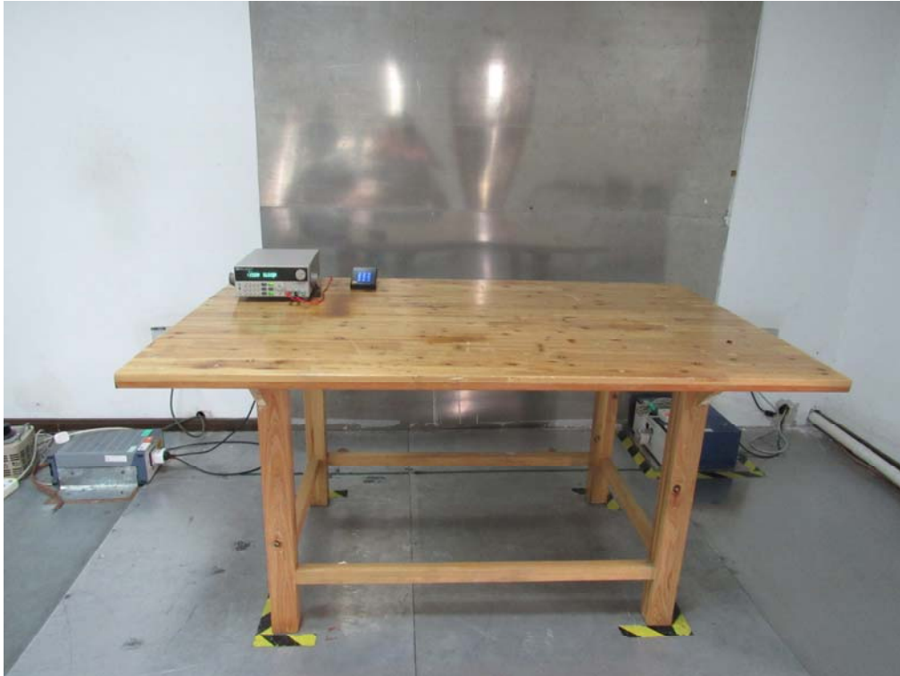
Conducted Emissions Setup Front View
