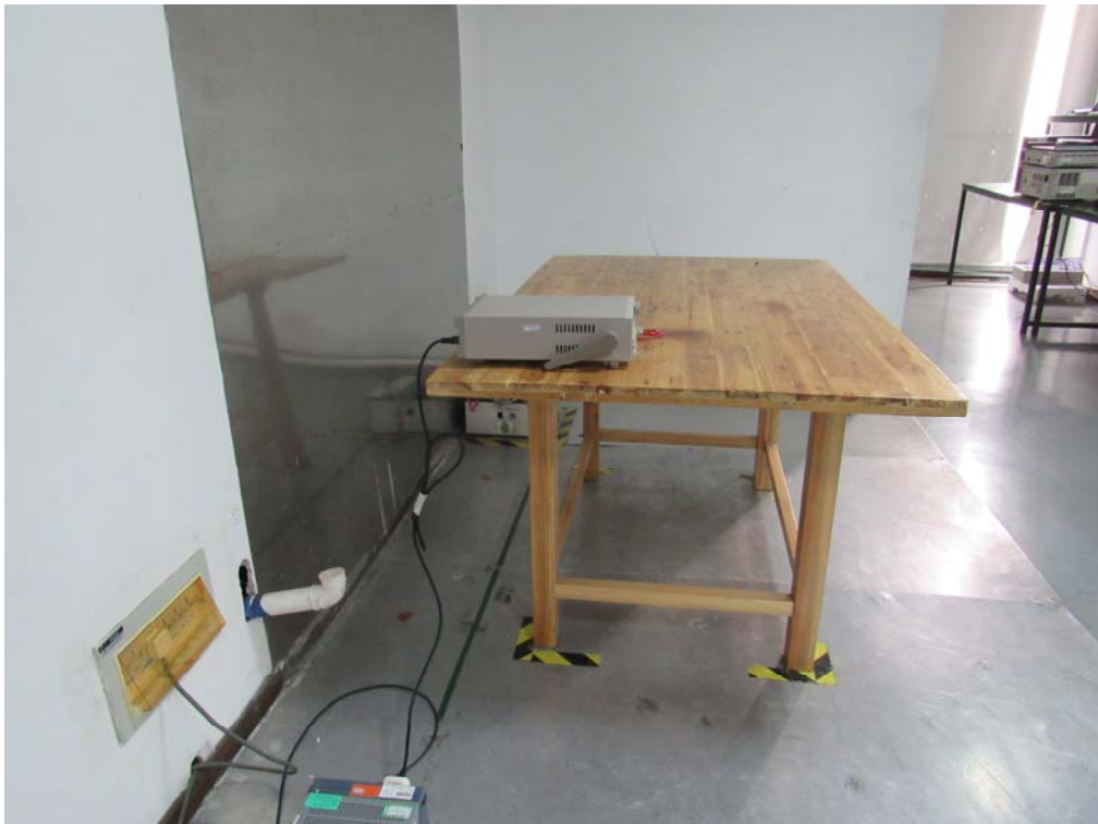
Conducted Emissions Setup Side View
