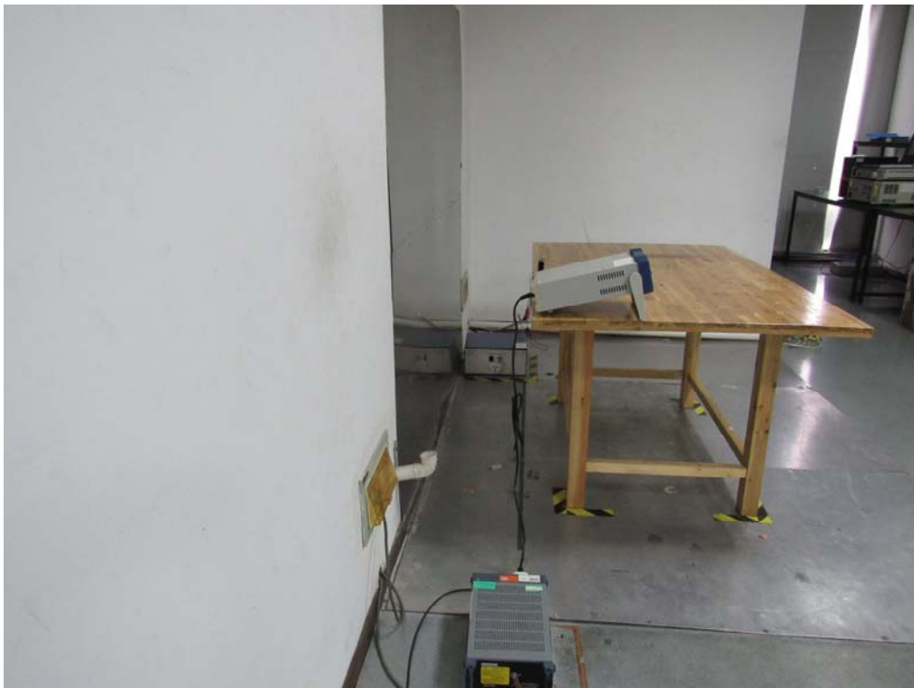
Conducted Emissions Setup Side View
