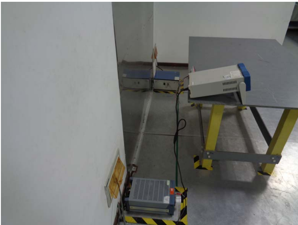
Conducted Emissions Setup Side View
