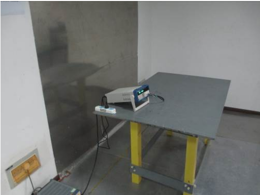
Conducted Emission Test Setup Side View
