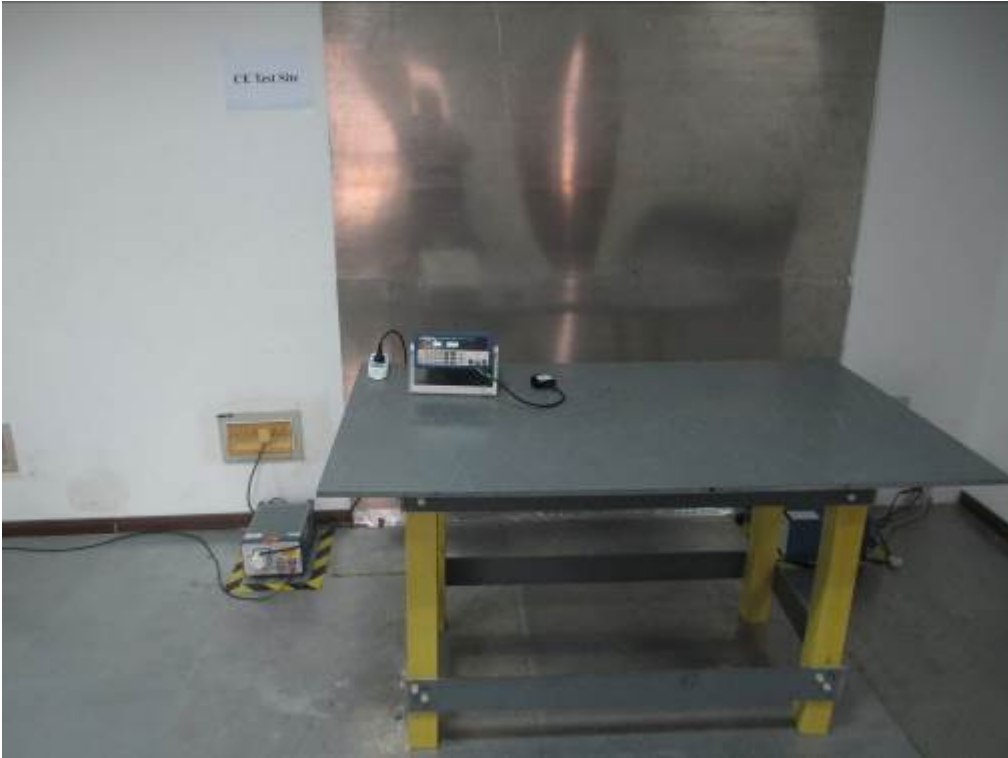
Conducted Emission Test Setup Front View
