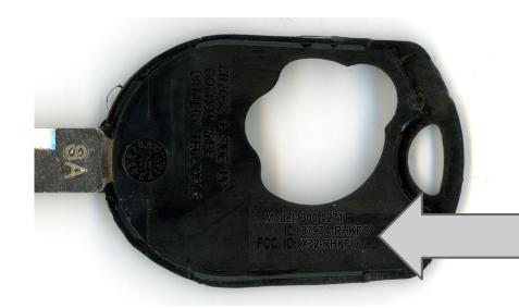
The FCC/IC label is located next to the battery under the back cover of the remote.
