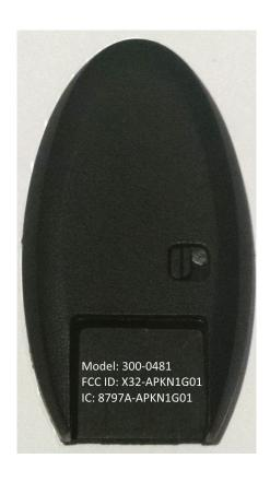
The FCC/IC label is located on the back of the remote shell beneath the emergency key.
