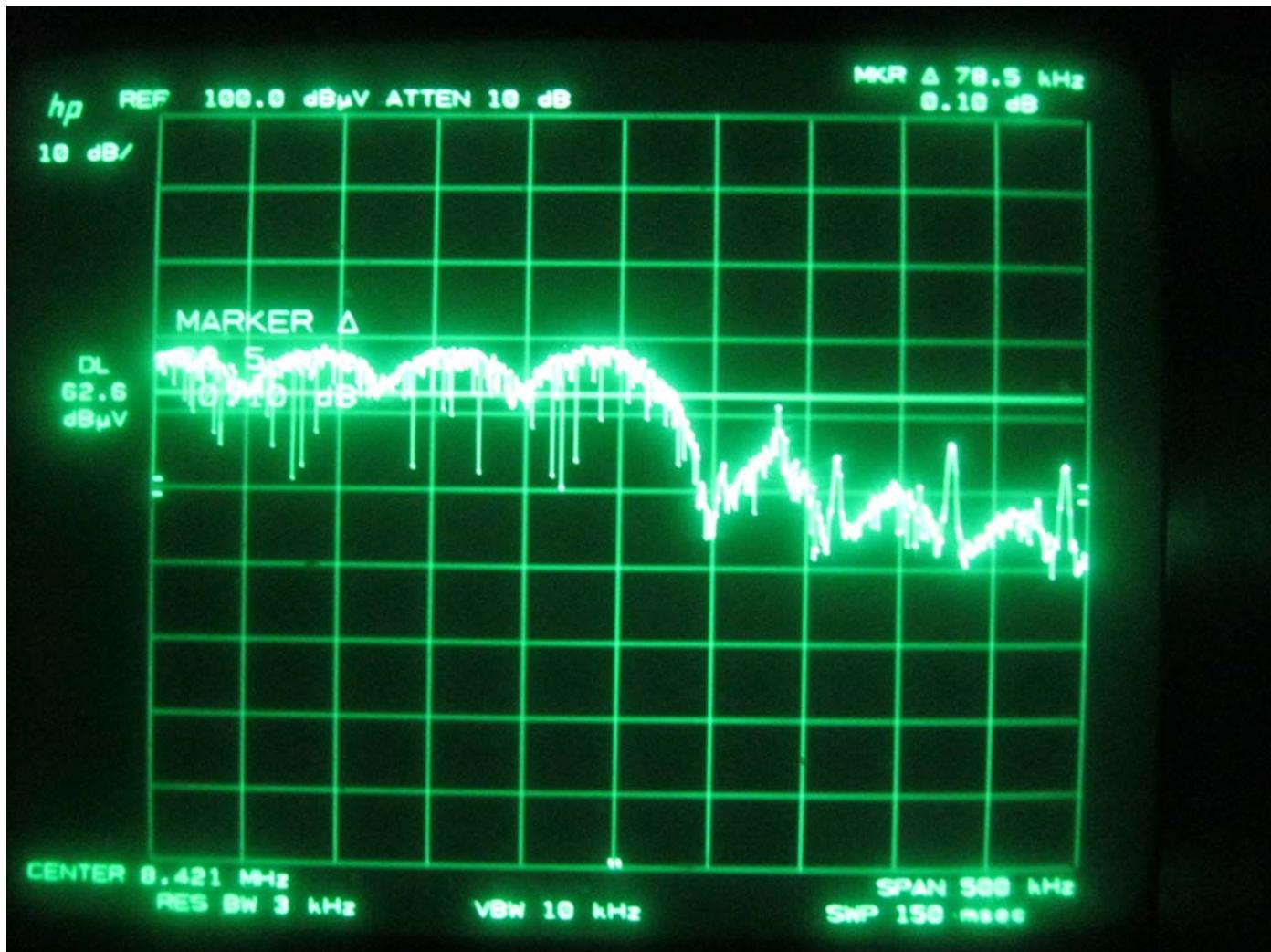
**-6 dB BANDWIDTH OF THE FUNDAMENTAL AT HIGH CHANNEL**
