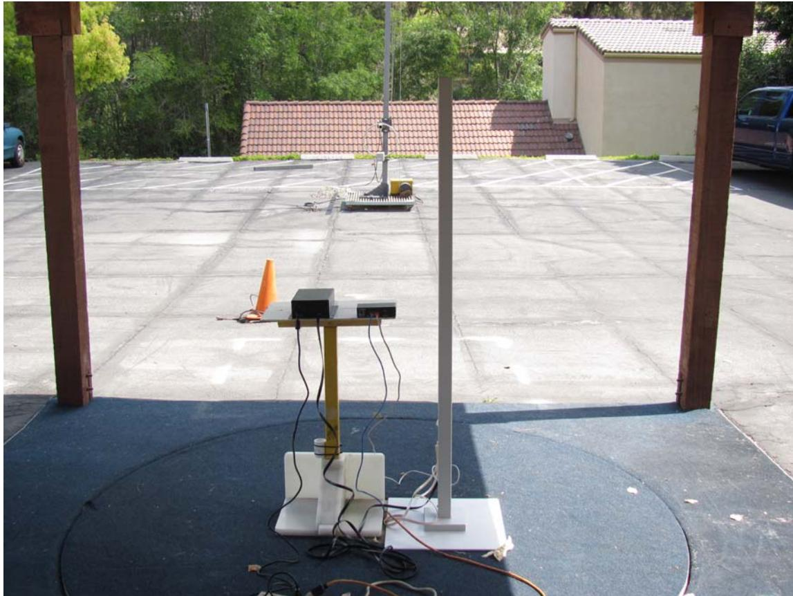
**FRONT VIEW****UNIVERSAL SURVEILLANCE SYSTEMS, LLC****58 kHz PEDESTAL SYSTEM****MODEL: USS-BLADE****FCC SUBPART B AND C – RADIATED EMISSIONS – BELOW 30 MHz****PHOTOGRAPH SHOWING THE EUT CONFIGURATION
