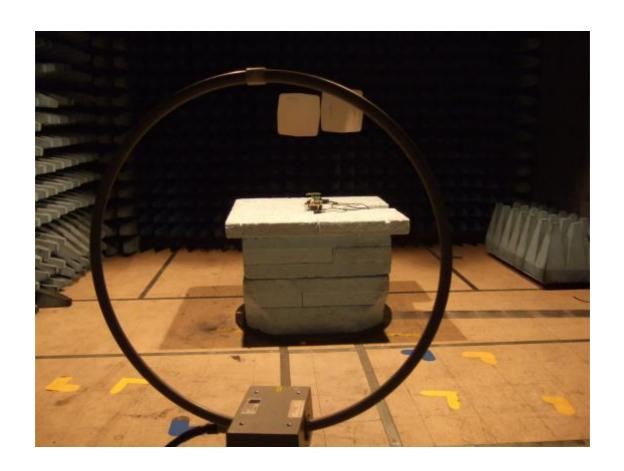
1.2 Test set-up, AC power line conducted emissions
