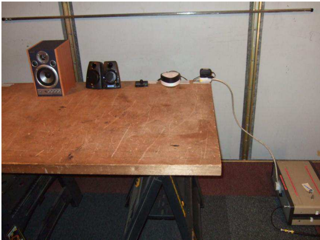
Photograph of the EUT as viewed from screened room (AC power line conducted emissions)
