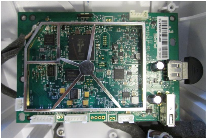
Main PCB Front without screening can
