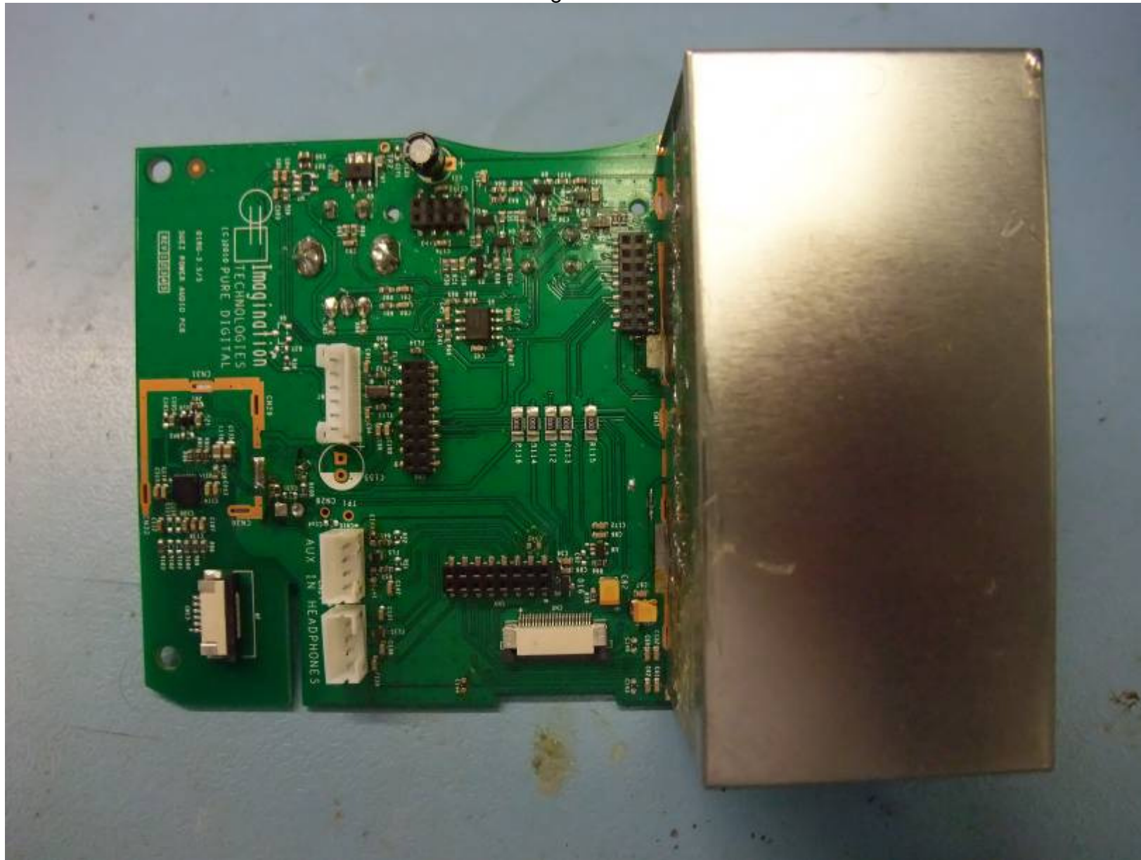
Main Power and Audio PCB – rear side with screening can fitted
