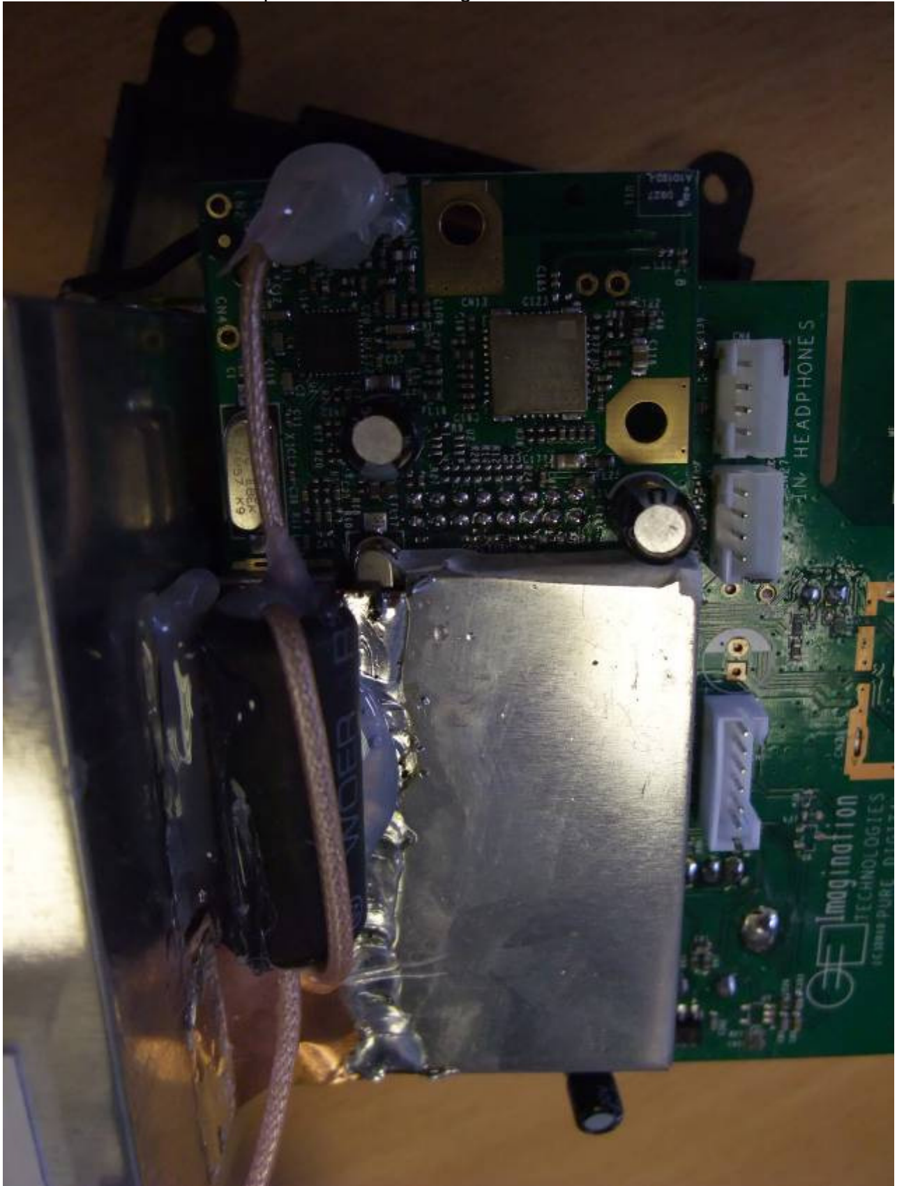
'Rufus' Main Module – top side with screening can fitted
