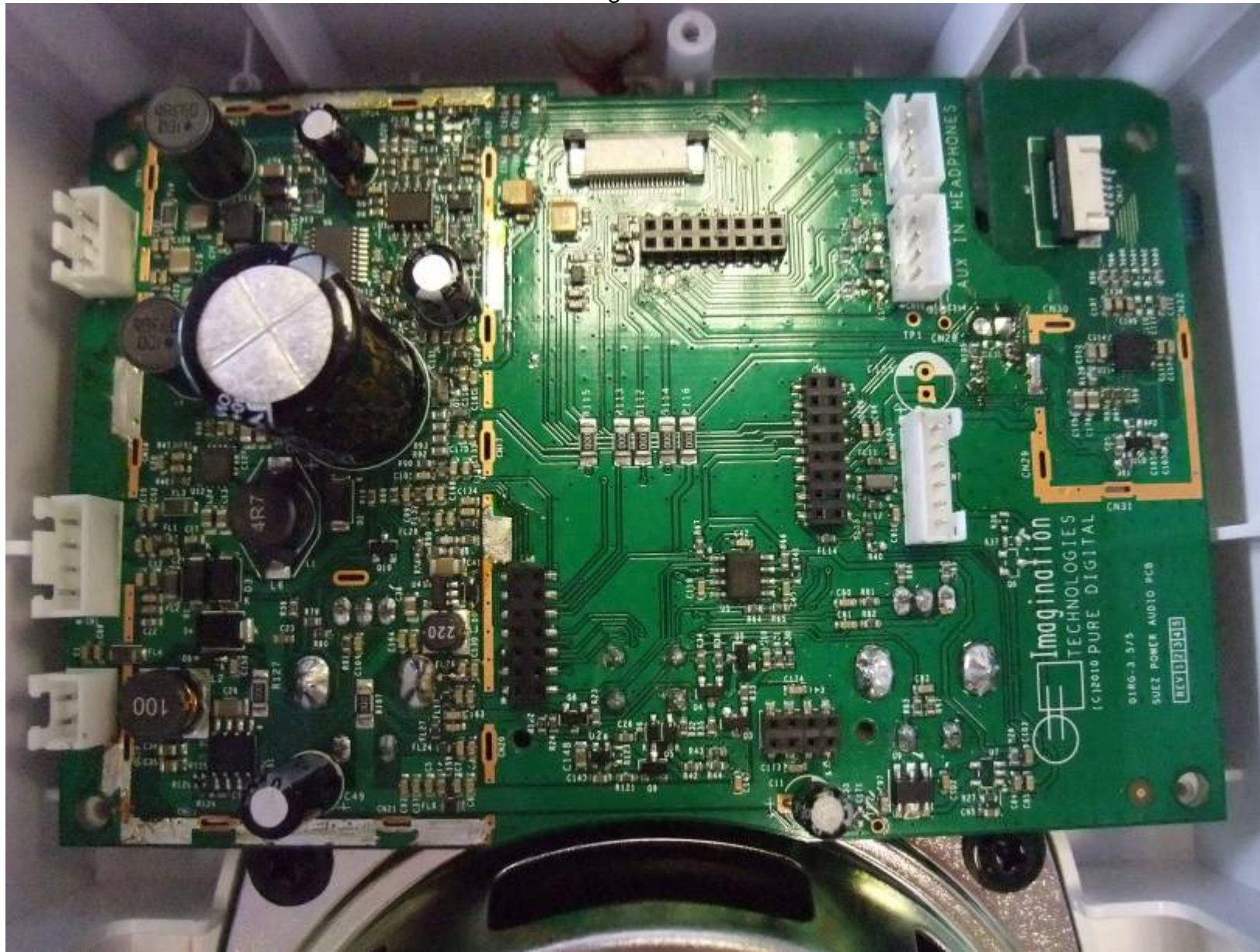
Main Power and Audio PCB – rear side with screening can removed
