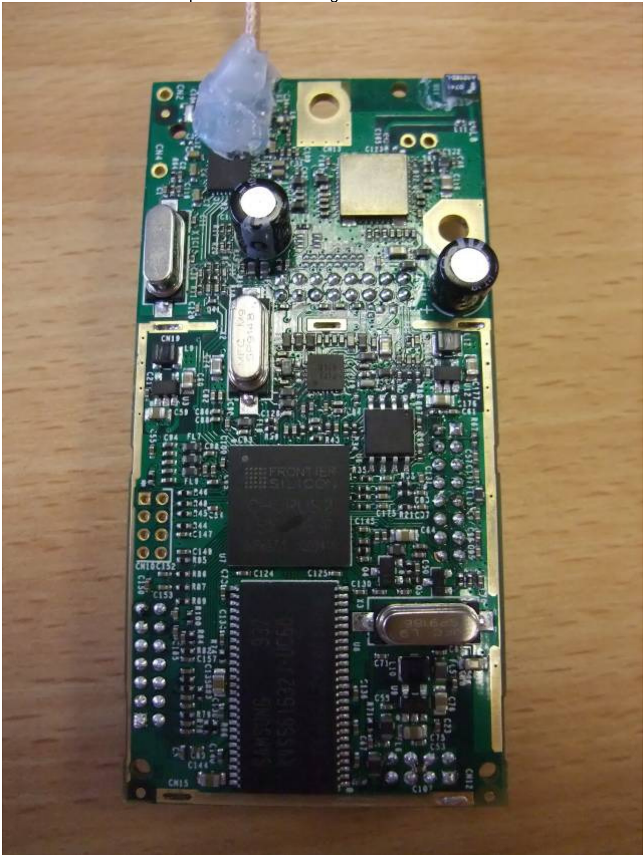
'Rufus' Main Module – top side with screening can removed
