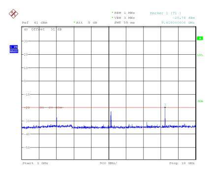
Note: Carrier Wave on all channels have been verified to be stronger than any individual modulated channel that would be evaluated for spurious emissions, thus reflecting worst-case compliance.
