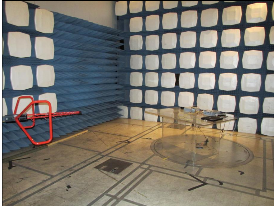
Photograph 2. Radiated Emissions, Test Setup, Below 1 GHz
