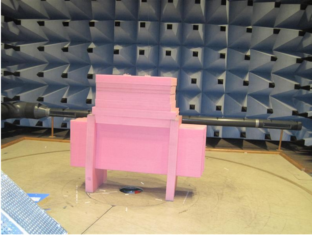
Photo Error! No text of specified style in document..9 Test setup regarding measurement of radiated emission, Rx, IC above 1 GHz.
