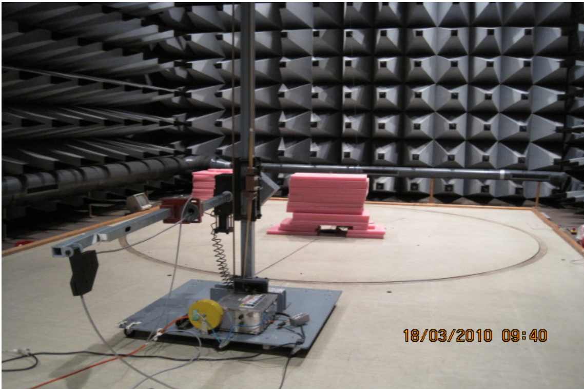
Photo 4.7.1 Test setup regarding measurement of field strength of fundamental.
