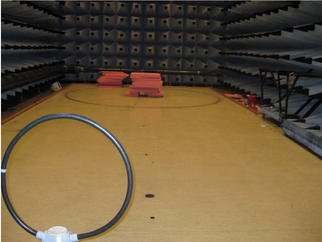
Photo Error! No text of specified style in document. 3 Test setup regarding measurement of radiated emission, 0.009-30 MHz.
