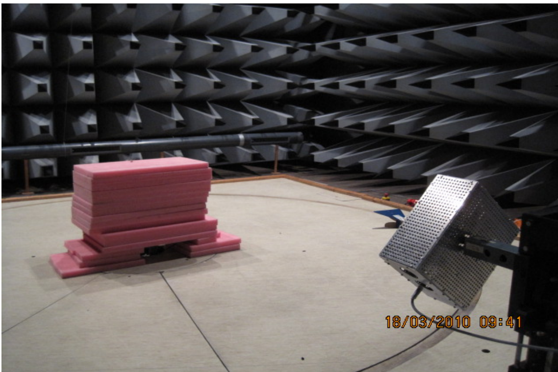
Photo 4.5.2 Test setup regarding measurement of radiated emission.
