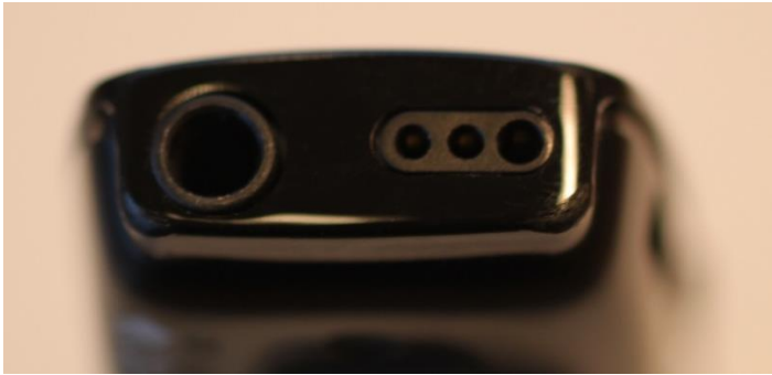
Bottom view (Left: line-in - right: FM/EURO Pin connector)
