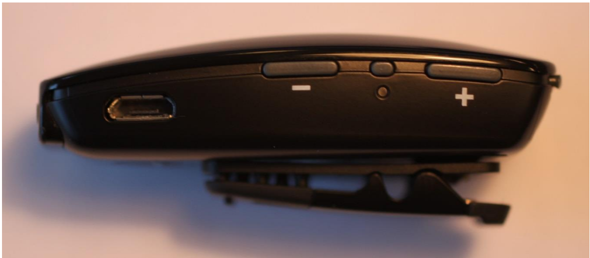
Right side view. (Micro USB, Volume down, Mute button/LED, Volume up)
