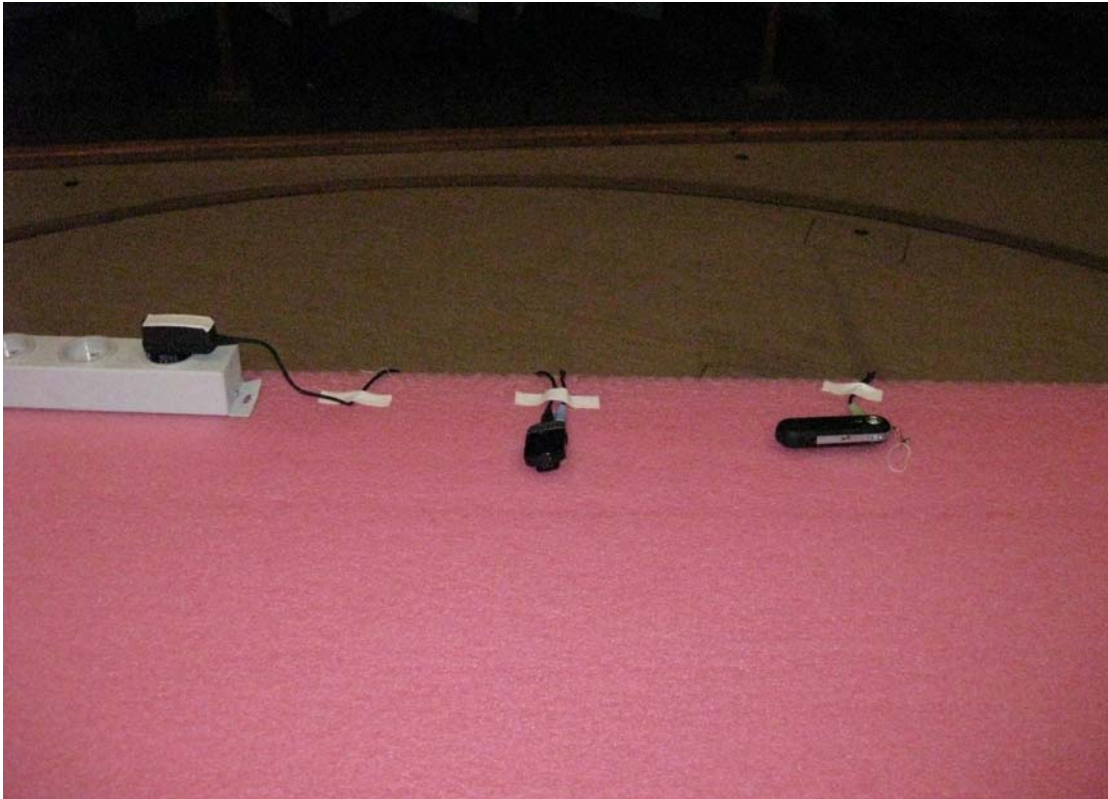
Photo 4.4.5 Test setup regarding measurement of radiated emission.
