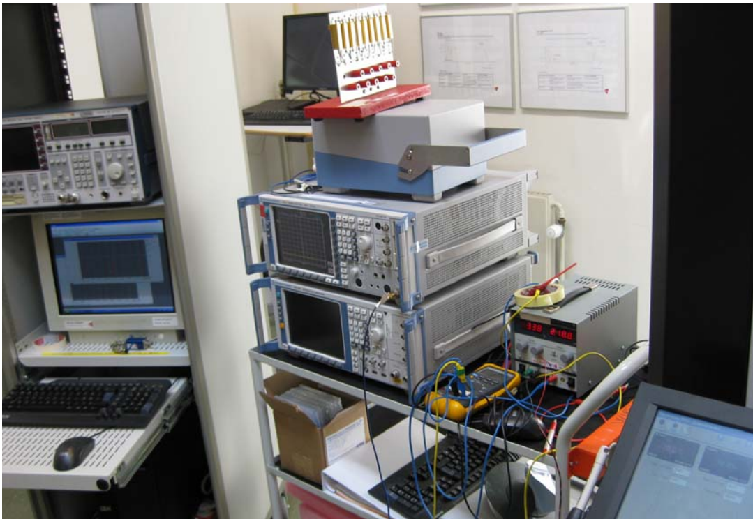
Photo 4.12.16 Test setup regarding measurement of occupied bandwidth, IC.
