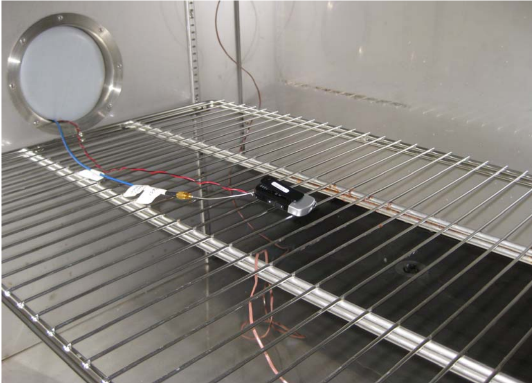
Photo 4.11.13 Test setup regarding measurement of band edge compliance of RF conducted emissions
