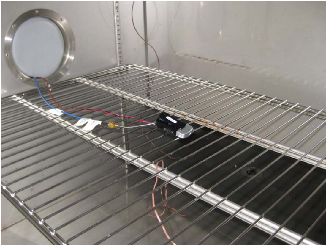
Photo 4.8.10 Test setup regarding measurement of time of occupancy (Dwell Time).
