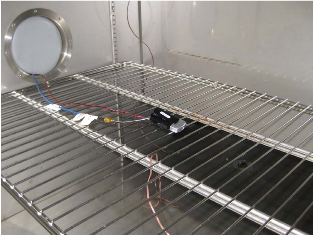
Photo 4.9.11 Test setup regarding measurement of peak output power, conducted.
