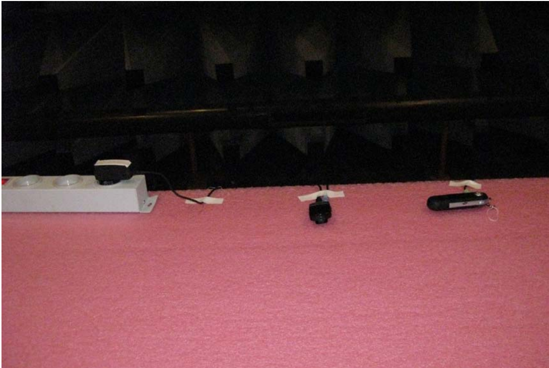
Photo 4.4.5 Test setup regarding measurement of radiated emission.
