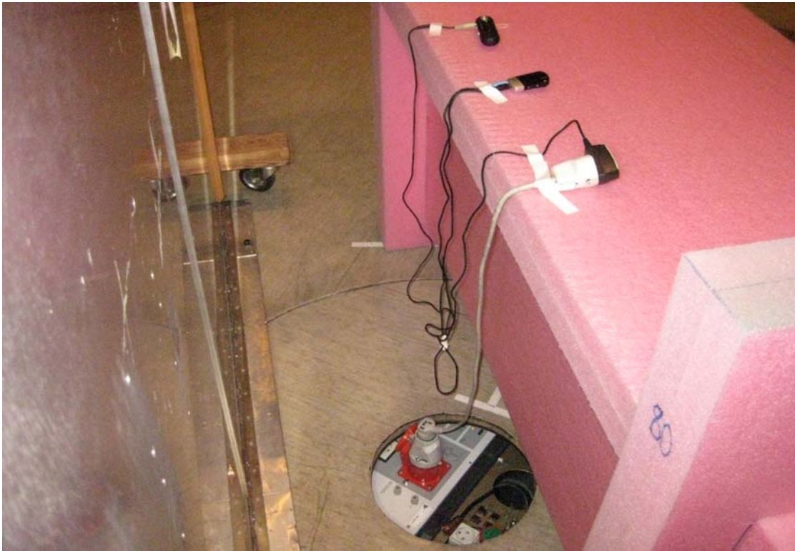
Photo Error! No text of specified style in document..1 Test setup regarding measurement of radio frequency voltage on mains.
