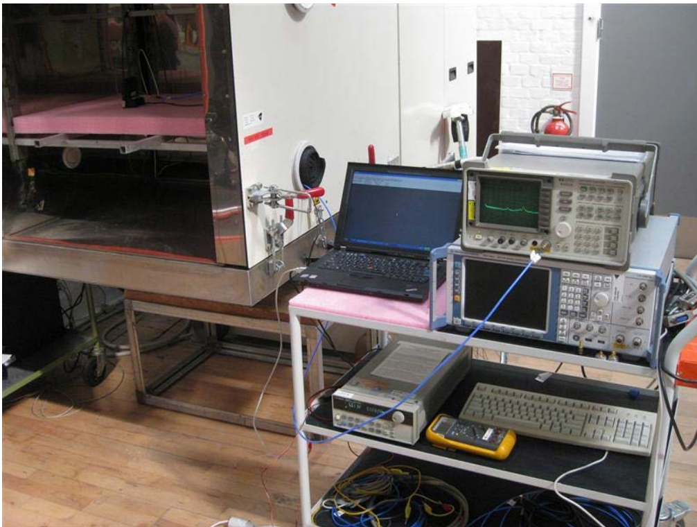
Photo 4.5.2 Test setup regarding measurement of maximum conducted output power.
