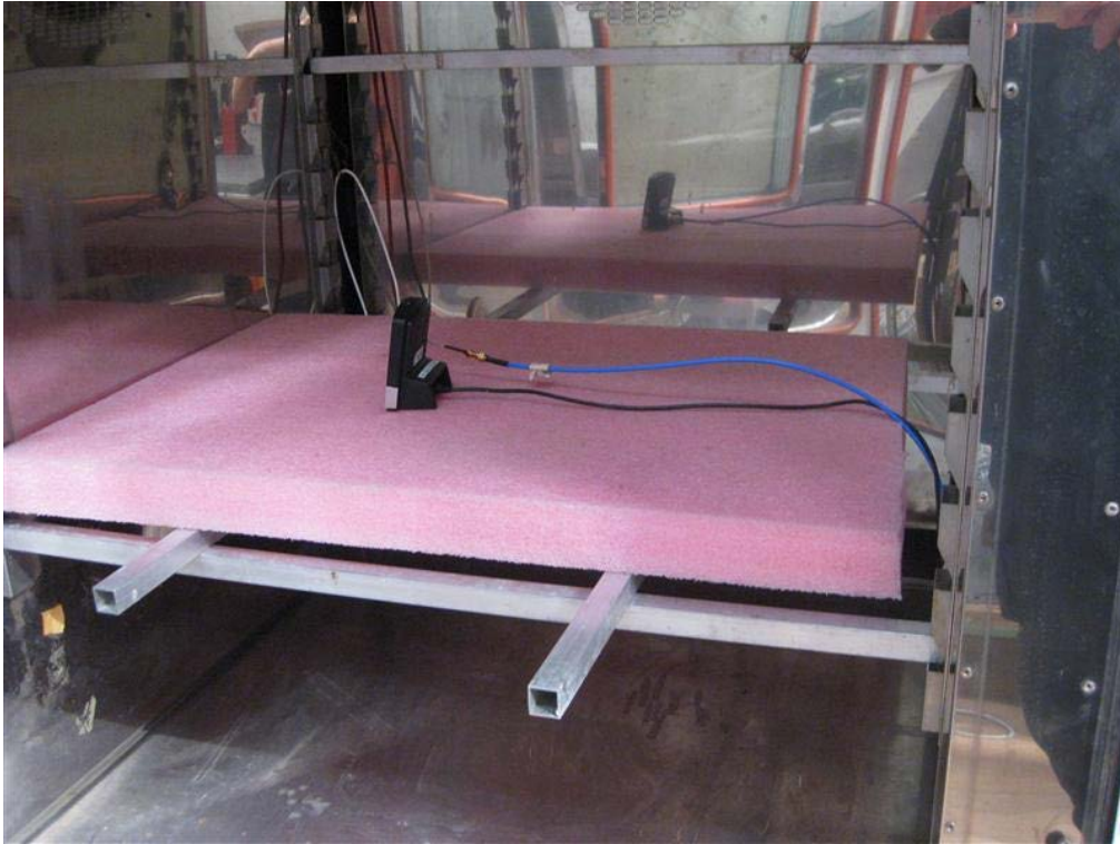
Photo 4.5.1 Test setup regarding measurement of maximum conducted output power.
