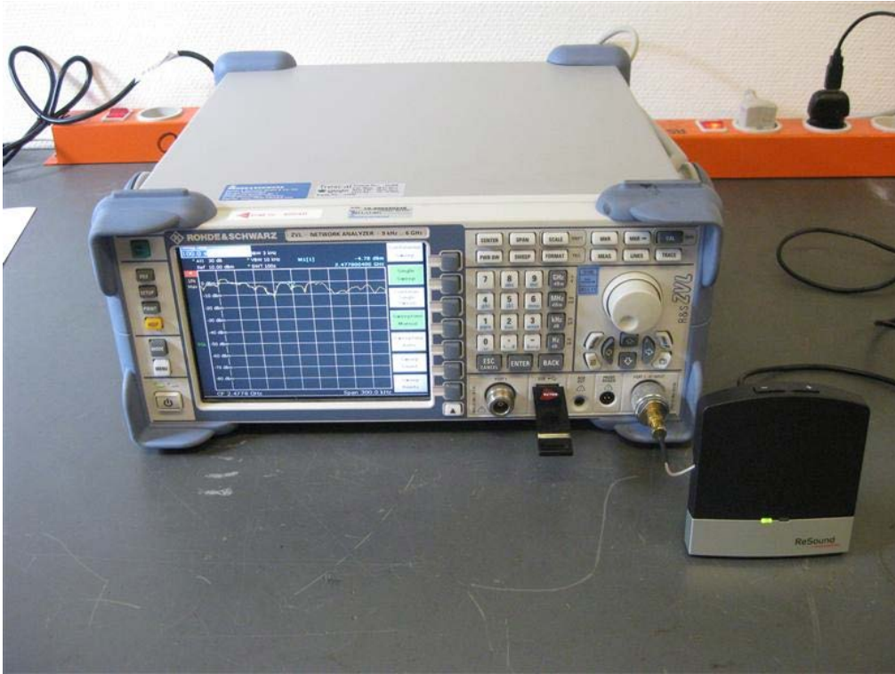
Photo 4.10.1 Test setup regarding measurement of power spectral density.
