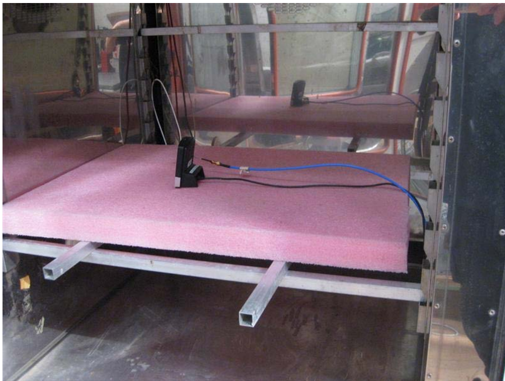
Photo 4.7.1 Test setup regarding measurement of 20 dB bandwidth.
