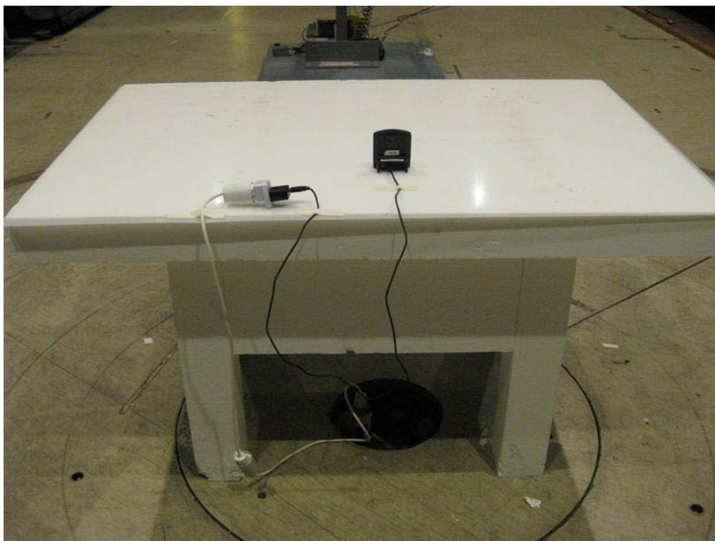
Photo 4.3.2 Test setup regarding measurement of radiated emission (below 1 GHz).
