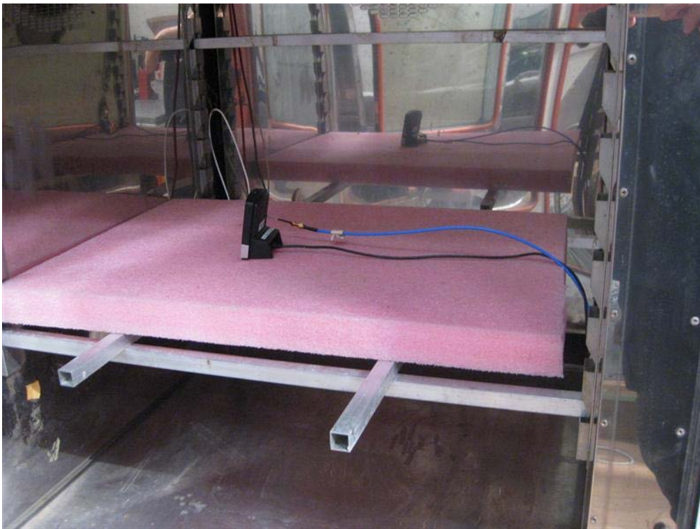
Photo 4.11.1 Test setup regarding measurement of occupied bandwidth, IC.
