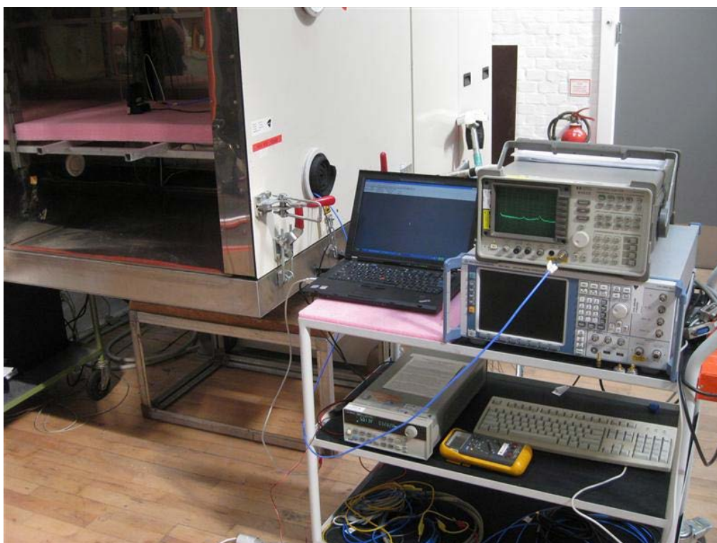
Photo 4.7.2 Test setup regarding measurement of 20 dB bandwidth.
