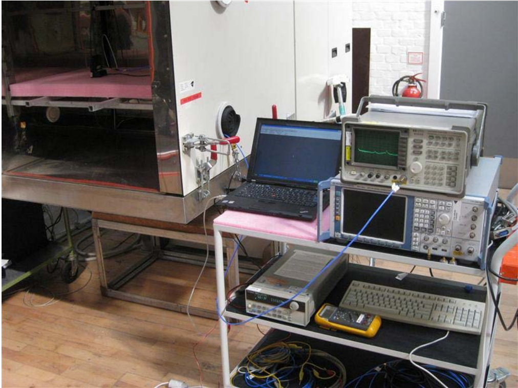
Photo 4.6.2 Test setup regarding measurement of 6 dB bandwidth.
