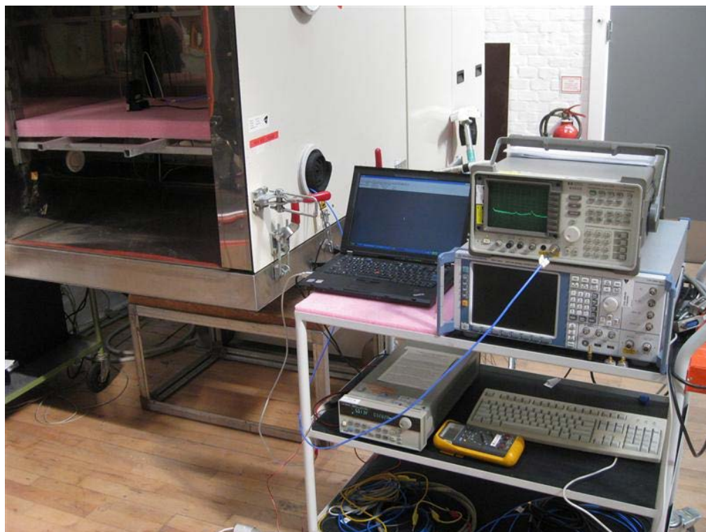
Photo 4.11.2 Test setup regarding measurement of occupied bandwidth, IC.
