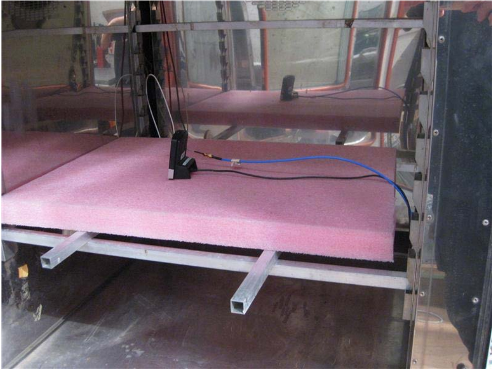
Photo 4.6.1 Test setup regarding measurement of 6 dB bandwidth.
