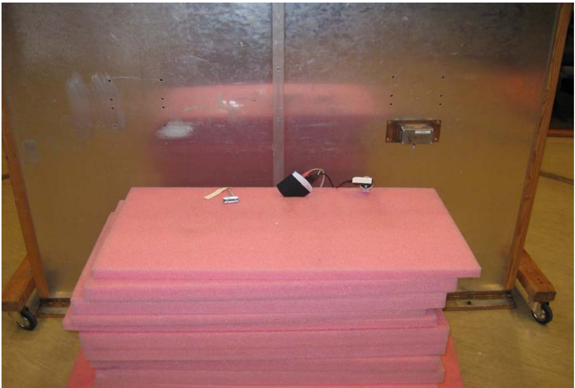
Photo 4.2.2 Test setup regarding measurement of radio frequency voltage on mains.
