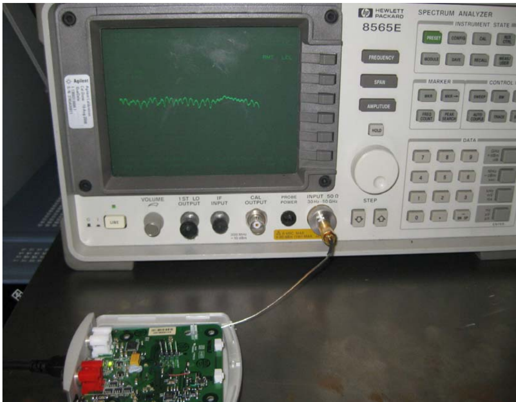
Photo 4.8.2 Test setup regarding measurement of conducted spurious emission.
