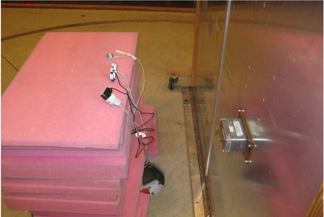
Photo 4.2.1 Test setup regarding measurement of radio frequency voltage on mains.
