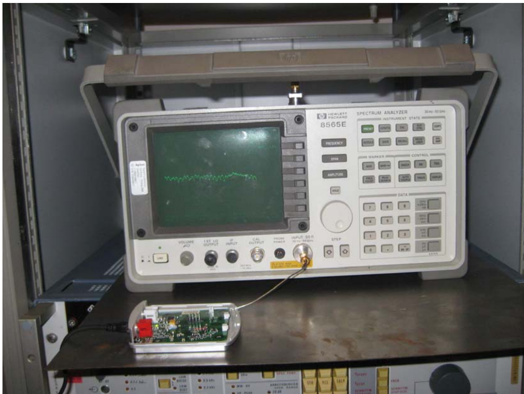
Photo 4.6.2 Test setup regarding measurement of the 6 dB bandwidth.
