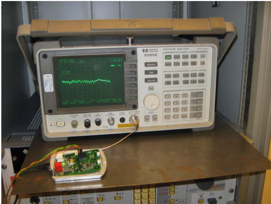
Photo 4.8.1 Test setup regarding measurement of conducted spurious emission.
