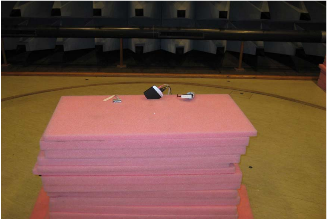
Photo 4.4.1 Test setup regarding measurement of radiated emission, 30 to 1000 MHz.
