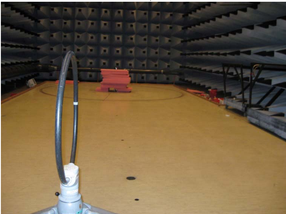
Photo Error! No text of specified style in document..2 Test setup regarding measurement of radiated emission, 0.009-30 MHz.
