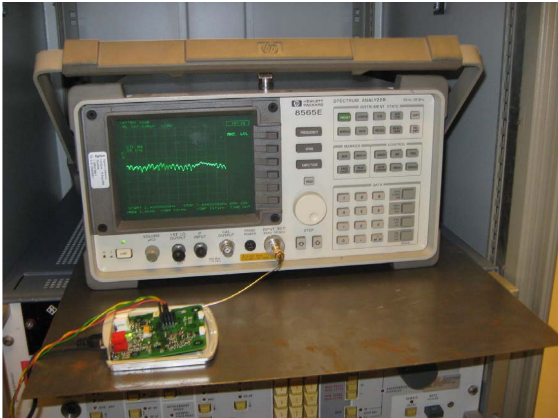
Photo 4.7.1 Test setup regarding measurement of conducted power output.
