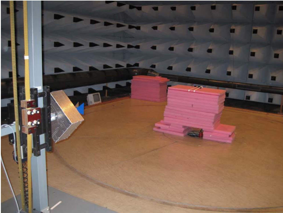
Photo 4.5.1 Test setup regarding measurement of radiated emission.
