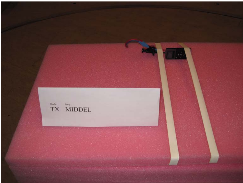
Photo 4.5.2 Test setup regarding measurement of radiated emission.
