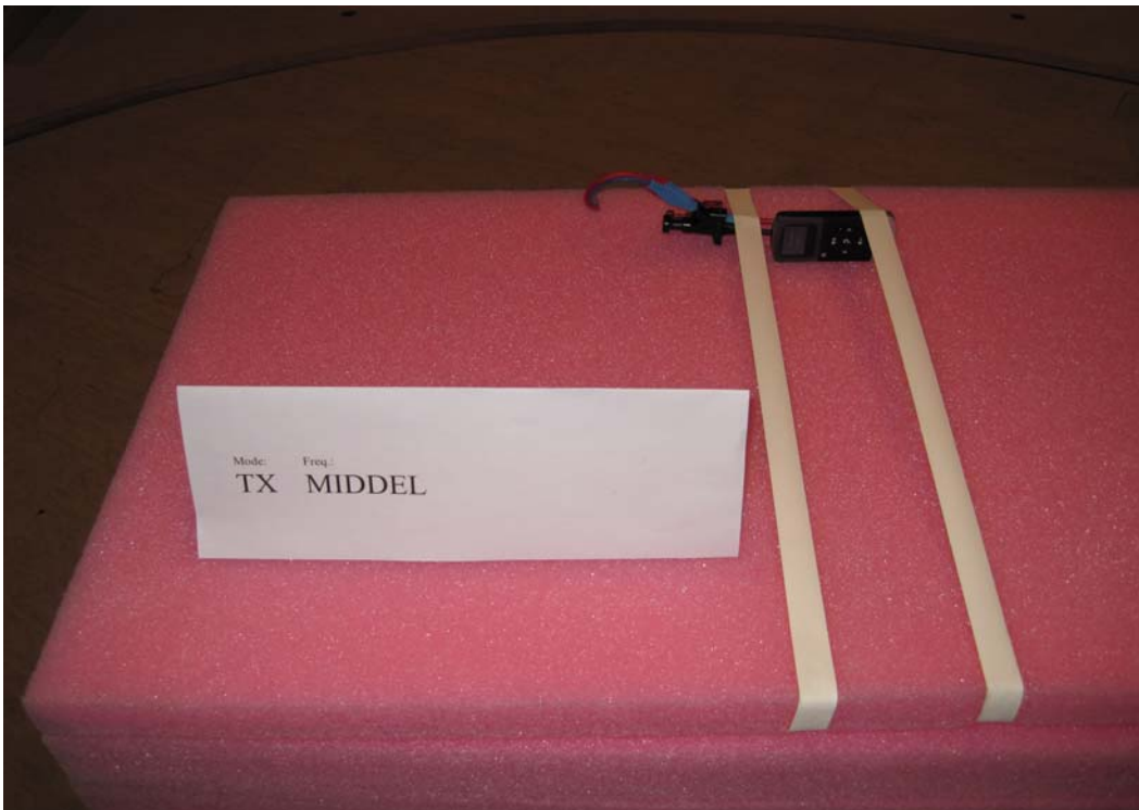
Photo 4.7.2 Test setup regarding measurement of field strength of fundamental.
