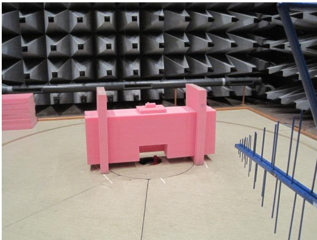
Photo 4.3.2 Test setup regarding measurement of radiated emission.
