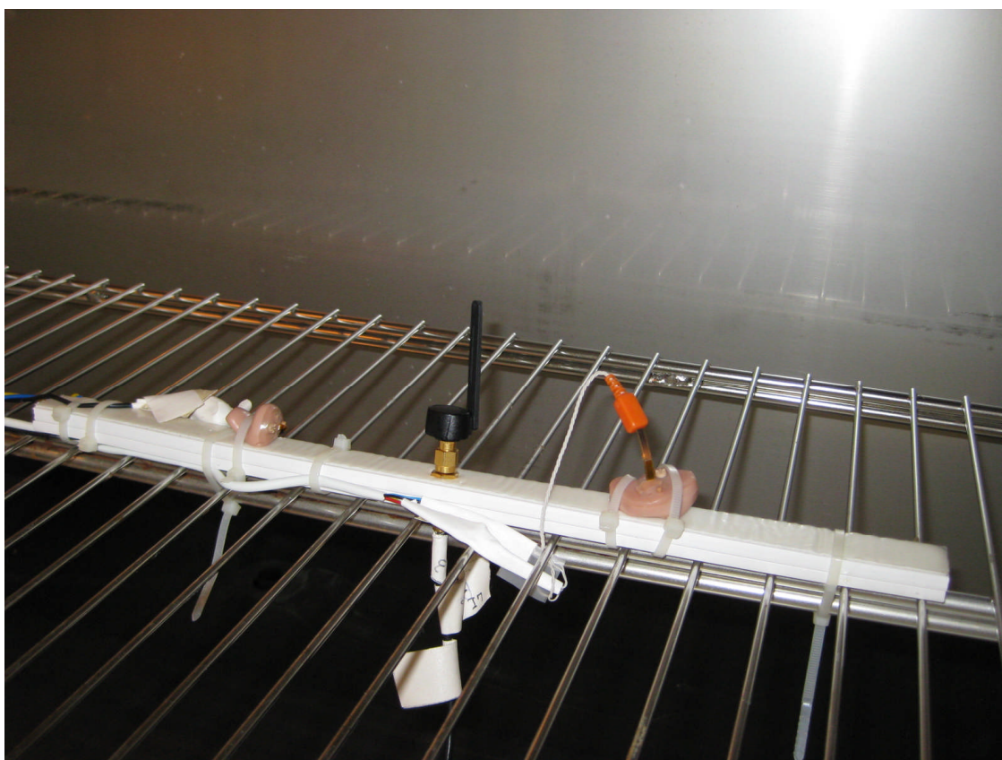
Photo 4.5.2 Test setup regarding measurement of 20 dB bandwidth.
