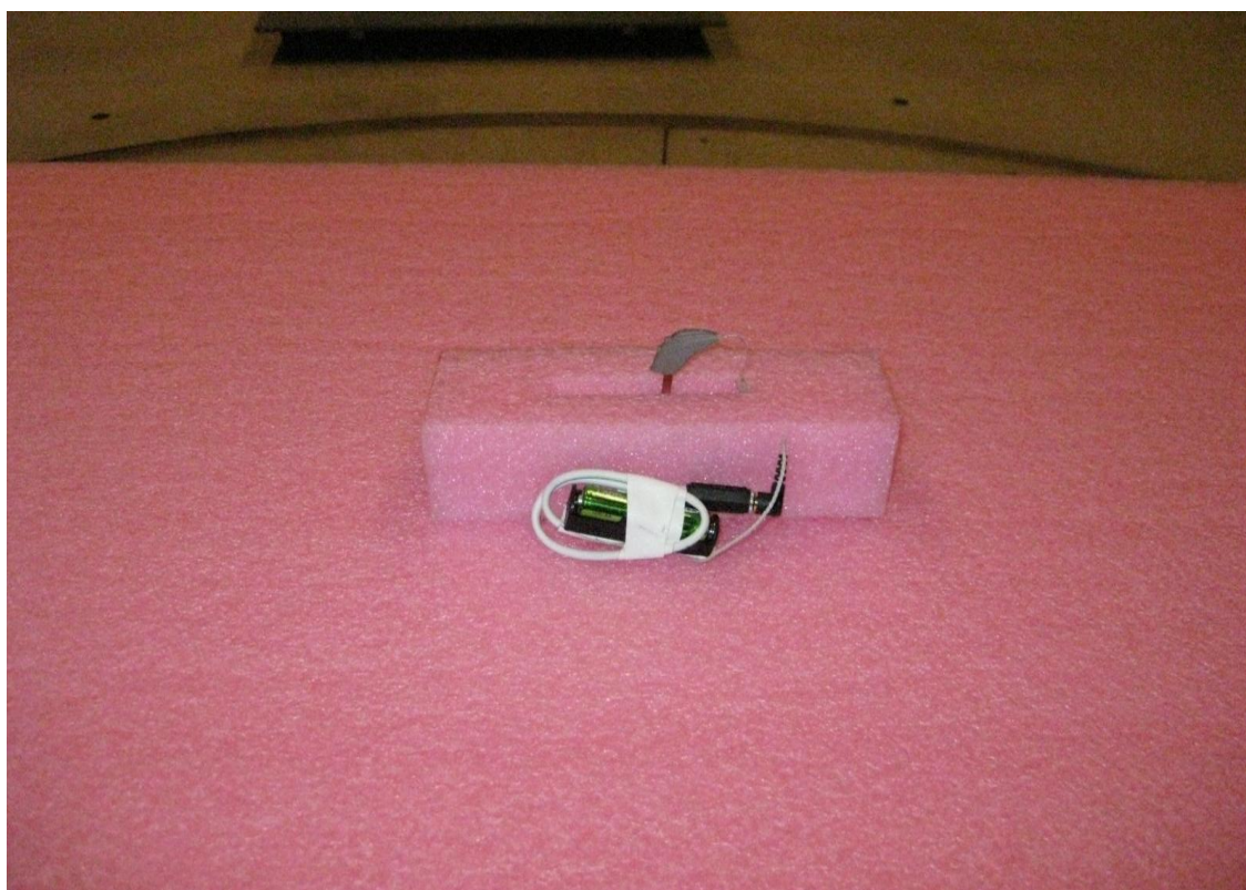
Photo 4.2.5 Test setup regarding measurement of radiated emission.
