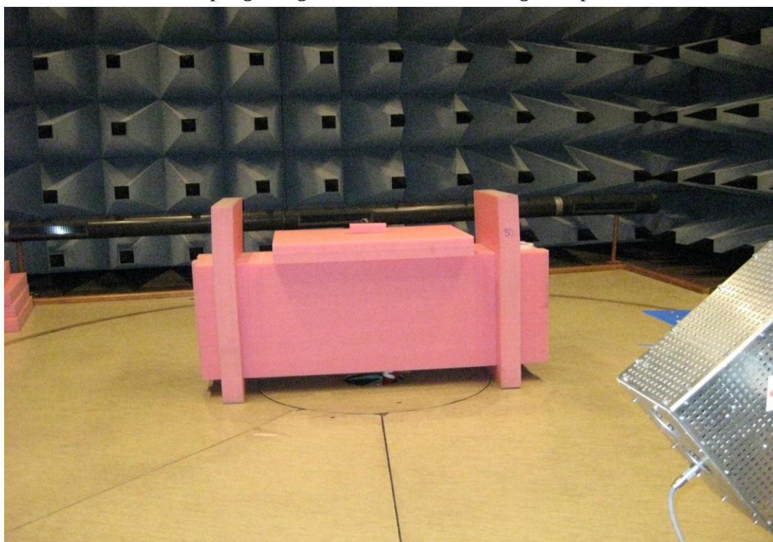
Photo 4.5.2 Test setup regarding measurement of band edge compliance.
