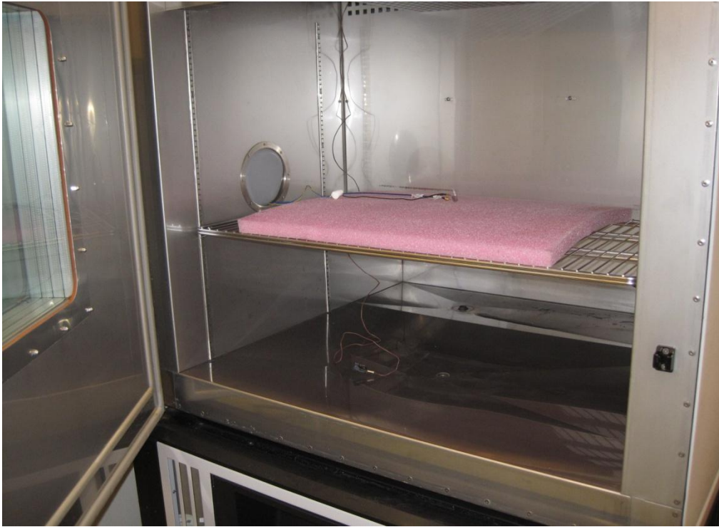
Photo 4.4.6 Test setup regarding measurement of 20 dB bandwidth.
