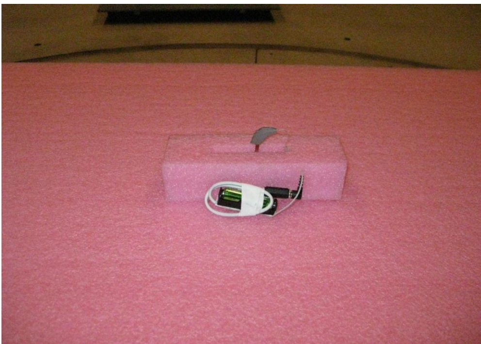
Photo 4.3.5 Test setup regarding measurement of field strength of fundamental.
