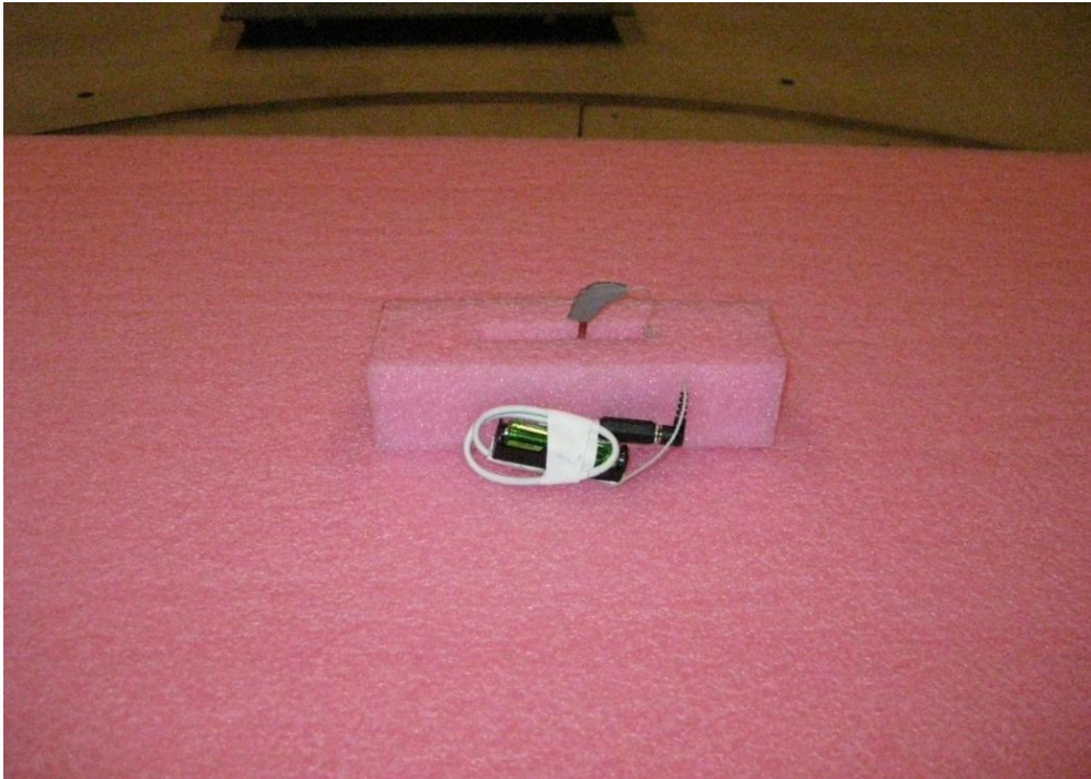
Photo 4.2.5 Test setup regarding measurement of radiated emission.
