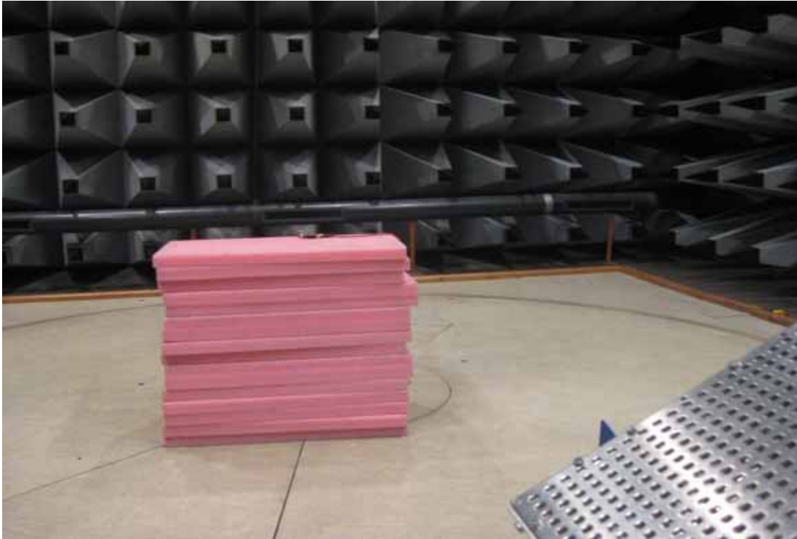
Photo 4.4.6 Test setup regarding measurement of radiated emission, 1 GHz to 25 GHz.
