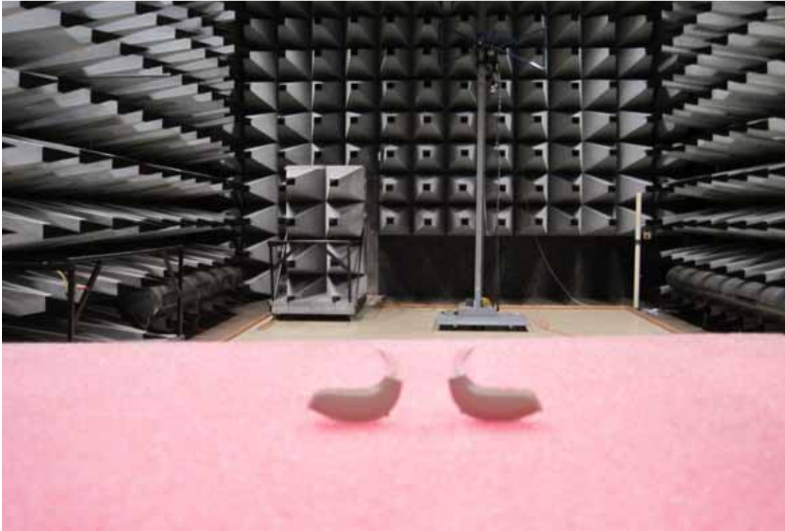
Photo 4.9.2 Test setup regarding measurement of radiated emission, Rx, IC, 30 MHz to 1000 MHz.
