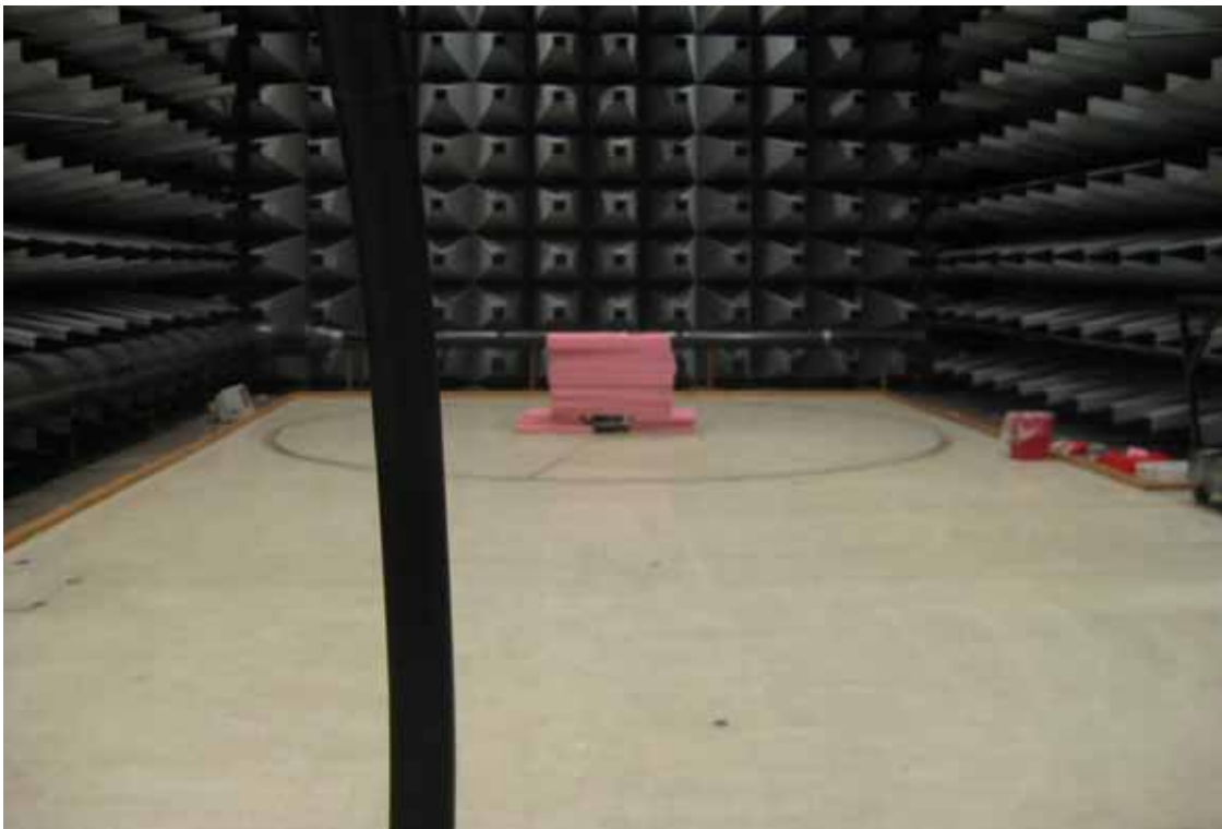
Photo 4.4.3 Test setup regarding measurement of radiated emission, 0.009 MHz - 30 MHz
