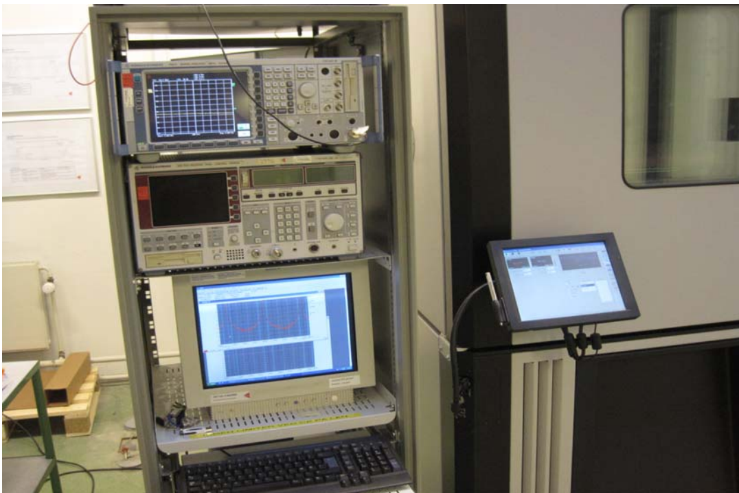
Photo 4.7.2 Test setup regarding measurement of occupied bandwidth, IC.
