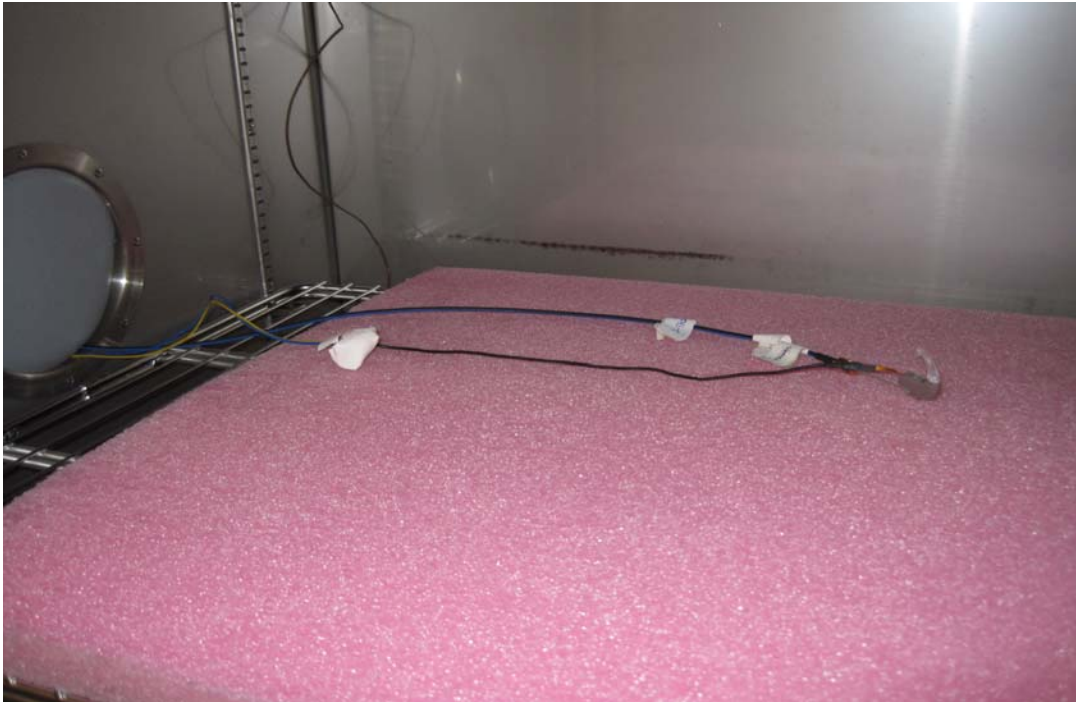
Photo 4.7.1 Test setup regarding measurement of occupied bandwidth, IC.
