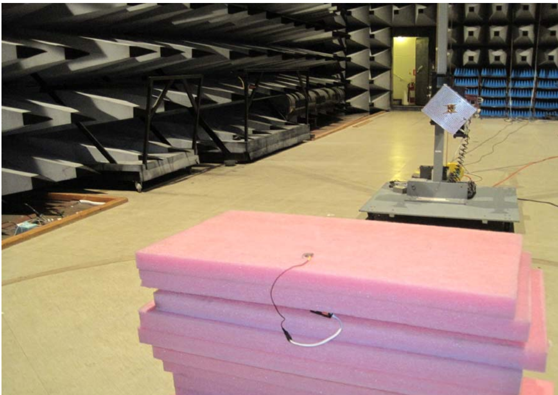
Photo 4.3.7 Test setup regarding measurement of radiated emission.
