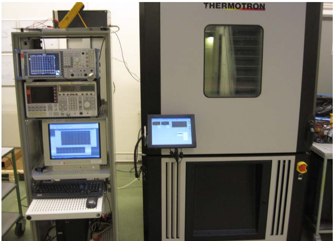
Photo 4.5.2 Test setup regarding measurement of 20 dB bandwidth.
