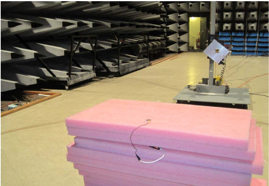
Photo 4.4.2 Test setup regarding measurement of field strength of fundamental.
