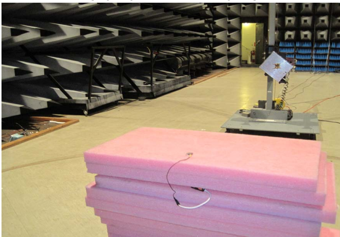
Photo 4.6.2 Test setup regarding measurement of band edge compliance.
