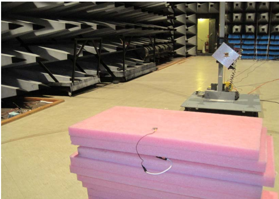
Photo 4.3.7 Test setup regarding measurement of radiated emission.
