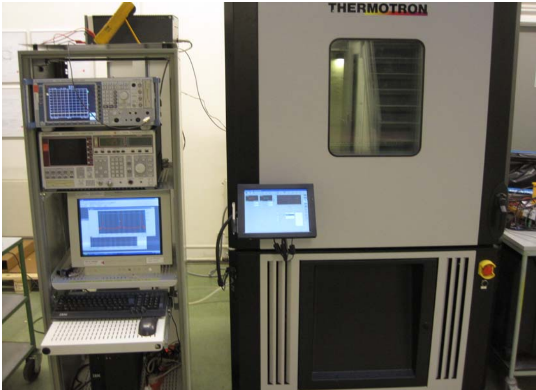
Photo 4.5.9 Test setup regarding measurement of 20 dB bandwidth.
