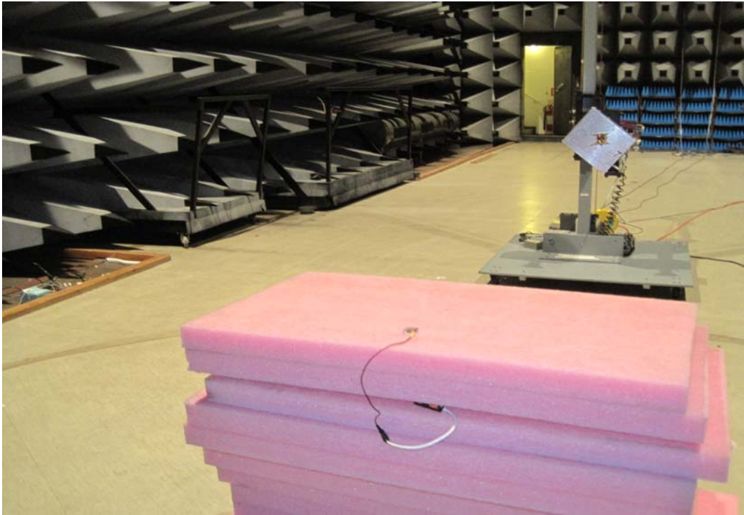
Photo 4.4.7 Test setup regarding measurement of field strength of fundamental.
