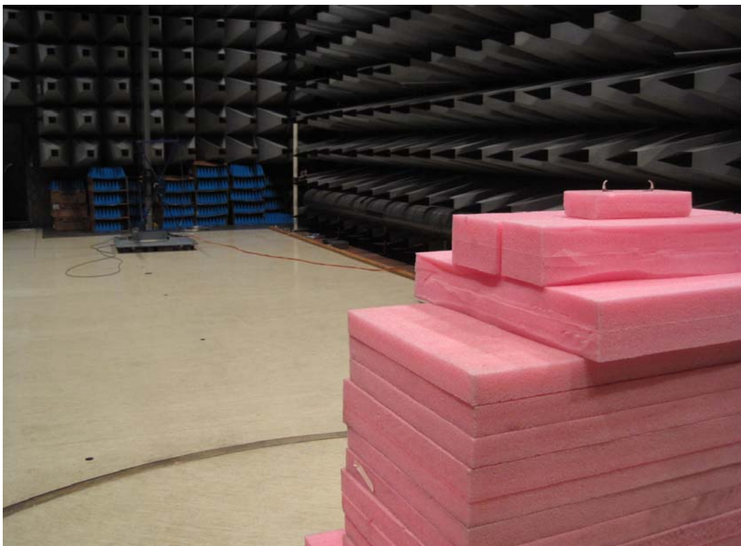
Photo 4.8.14 Test setup regarding measurement of radiated emission, Rx, IC.
