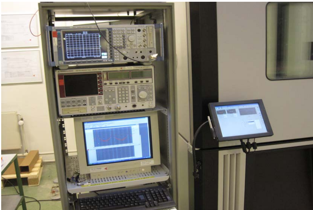
Photo 4.7.13 Test setup regarding measurement of occupied bandwidth, IC.
