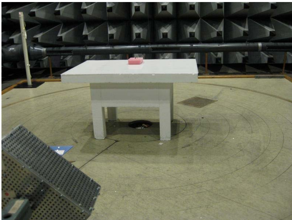
Photo 4.9.1 Test setup regarding measurement of field strength of fundamental.
