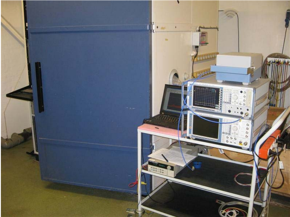
Photo 4.10.2 Test setup regarding measurement of 20 dB bandwidth
