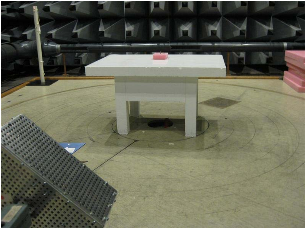
Photo 4.7.1 Test setup regarding measurement of field strength of fundamental.
