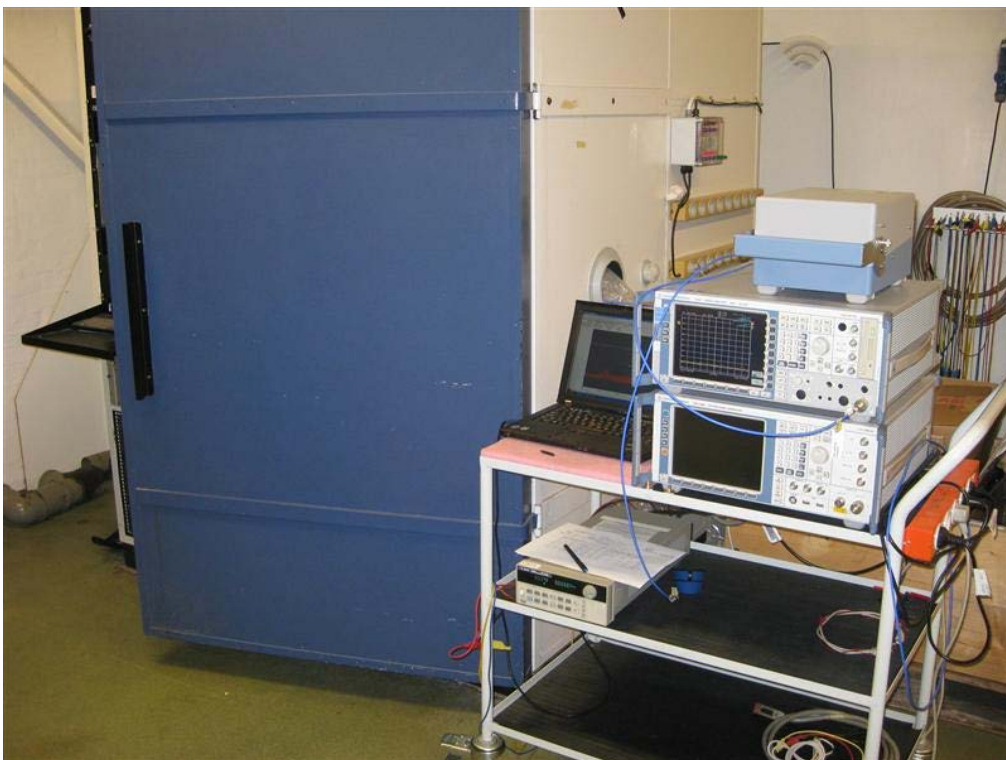
Photo 4.11.2 Test setup regarding measurement of band edge compliance.
