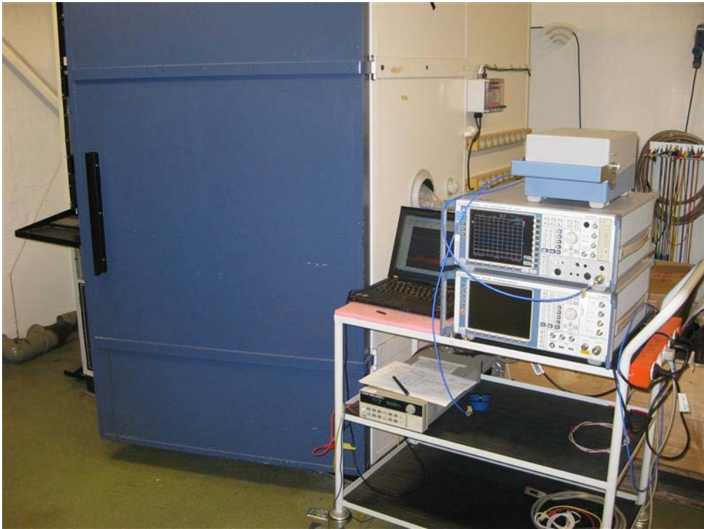
Photo 4.9.2 Test setup regarding measurement of 20 dB bandwidth
