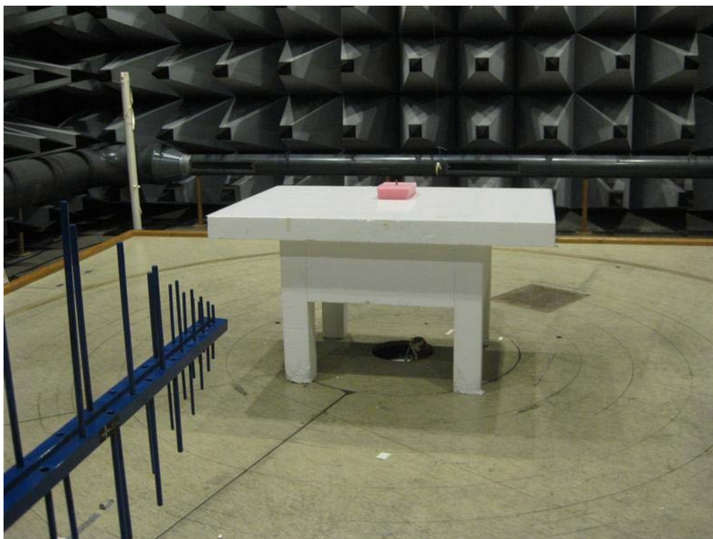
Photo 4.3.1 Test setup regarding measurement of radiated emission (below 1 GHz).
