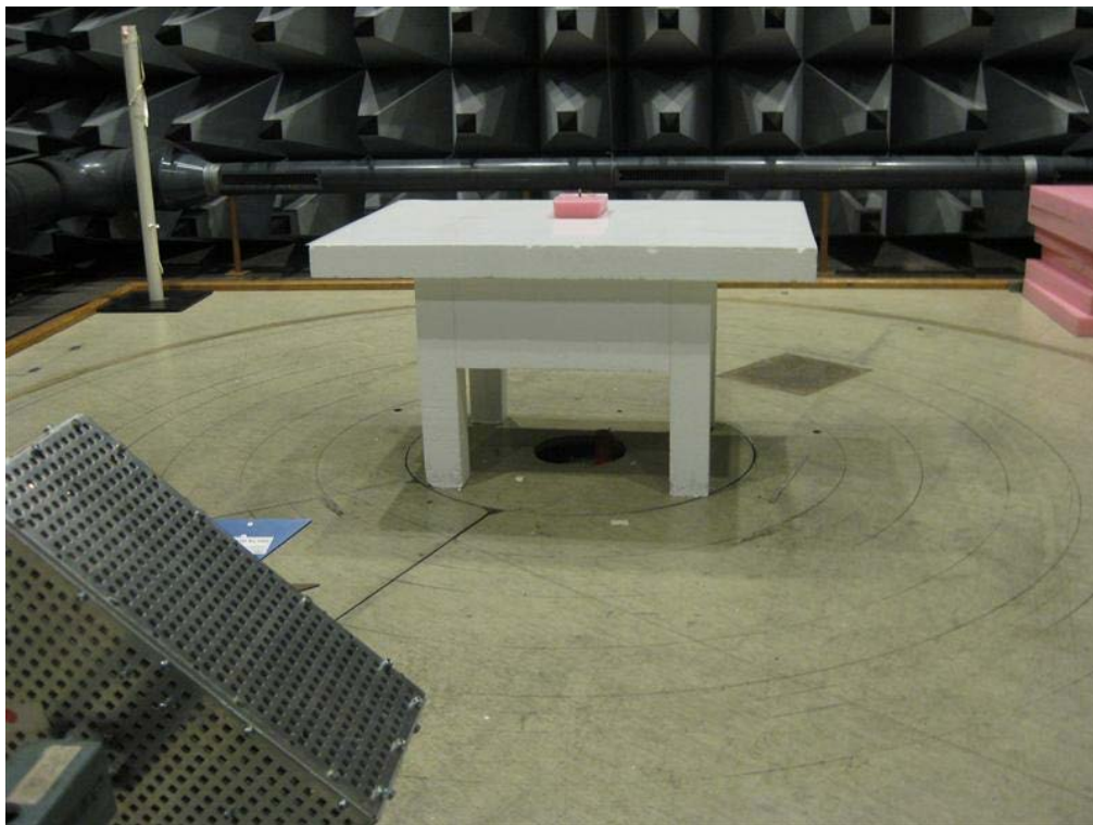
Photo 4.5.1 Test setup regarding measurement of radiated emission (above 1 GHz)
