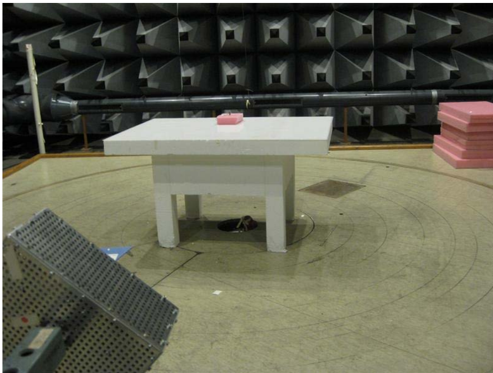
Photo 4.8.1 Test setup regarding measurement of field strength of fundamental.
