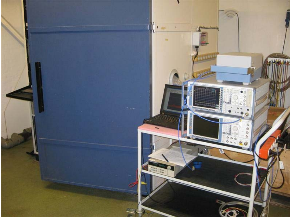
Photo 4.9.2 Test setup regarding measurement of 20 dB bandwidth
