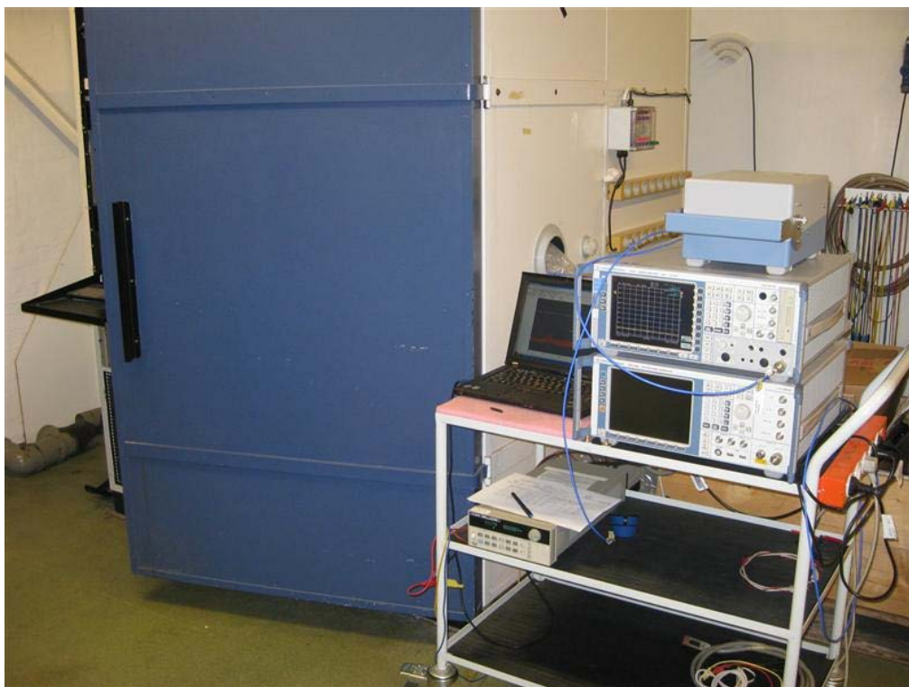
Photo 4.10.2 Test setup regarding measurement of 20 dB bandwidth
