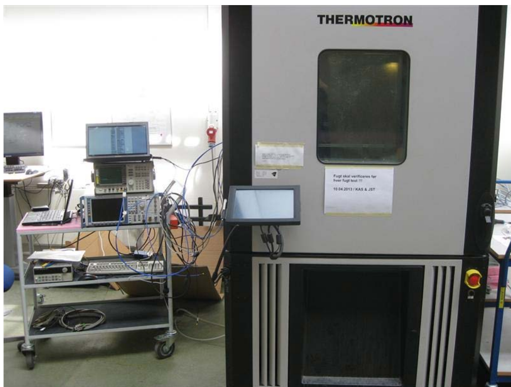
Photo 4.14.1 Test setup regarding measurement of 20 dB bandwidth.
