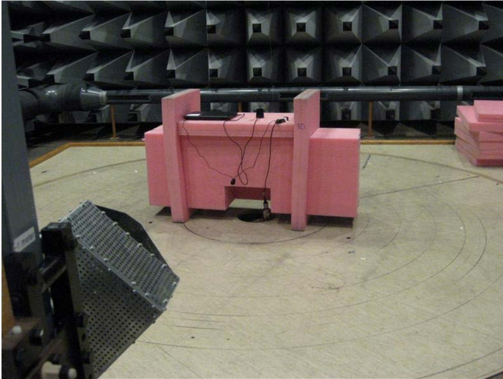
Photo 4.11.1 Test setup regarding measurement of field strength of fundamental.
