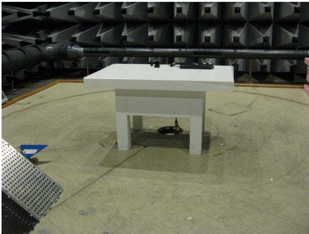
Photo 4.10.1 Test setup regarding measurement of radiated emission above 1 GHz.
