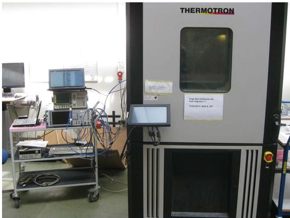
Photo 4.19.1 Test setup regarding occupied bandwidth.
