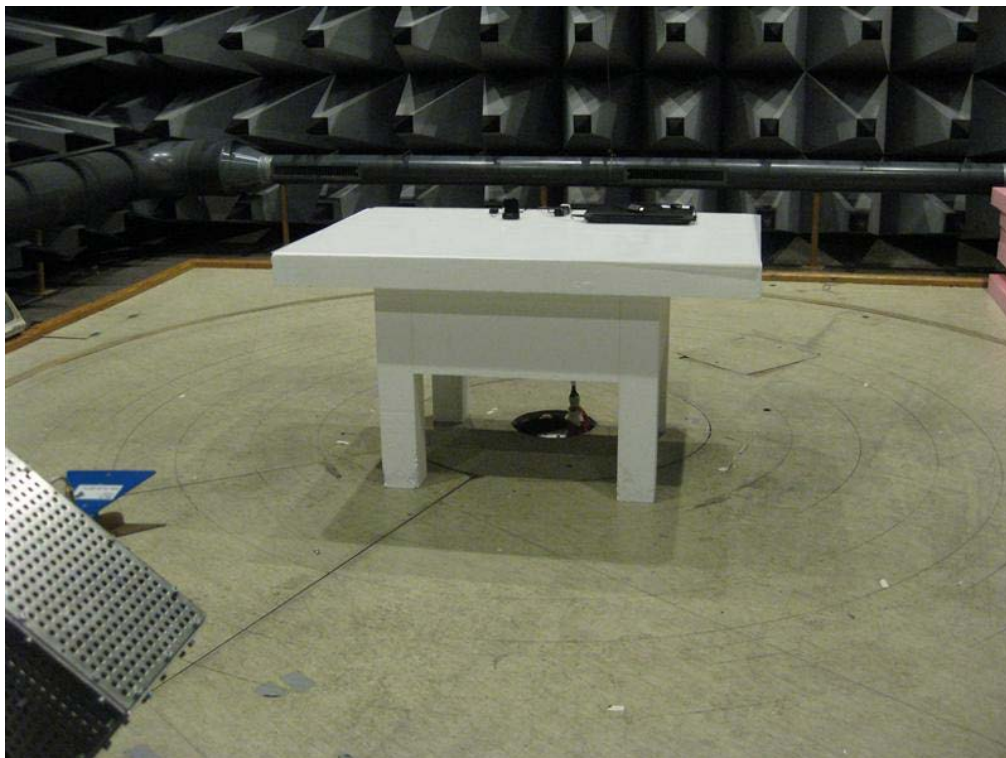
Photo 4.12.1 Test setup regarding measurement of field strength of fundamental.
