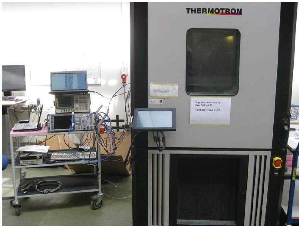
Photo 4.13.1 Test setup regarding measurement of 20 dB bandwidth.
