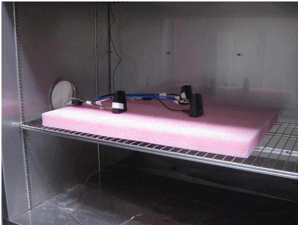
Photo 4.14.2 Test setup regarding measurement of 20 dB bandwidth.
