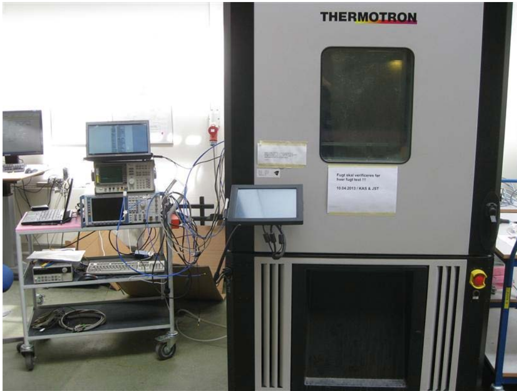
Photo 4.14.1 Test setup regarding measurement of 20 dB bandwidth.
