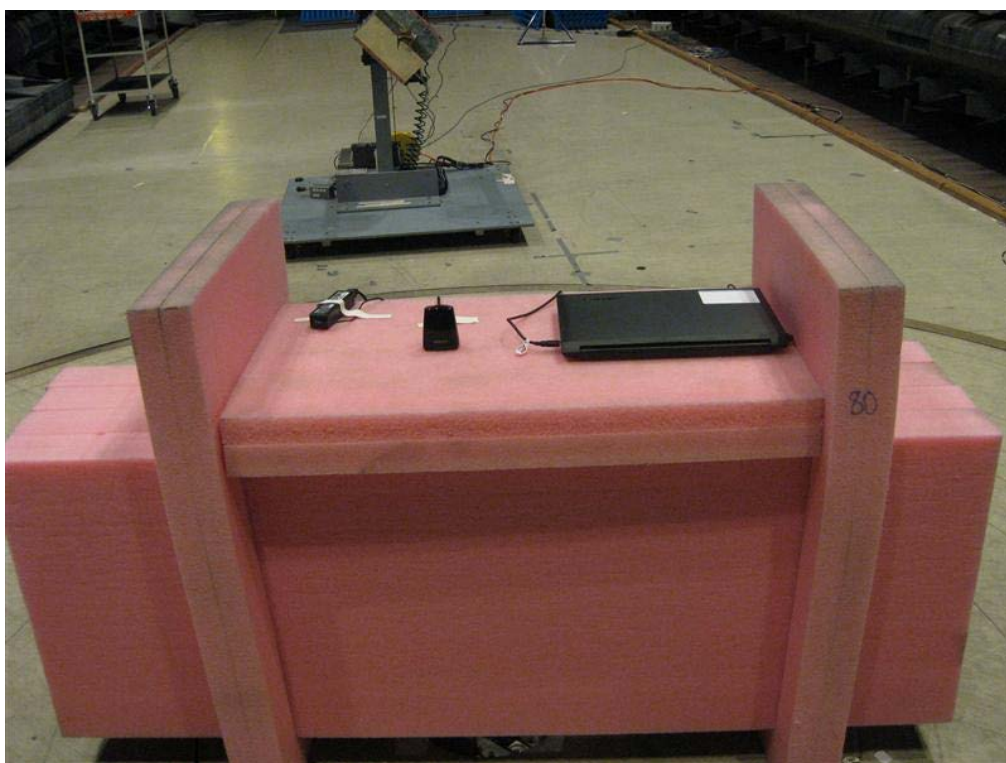
Photo 4.11.2 Test setup regarding measurement of field strength of fundamental.
