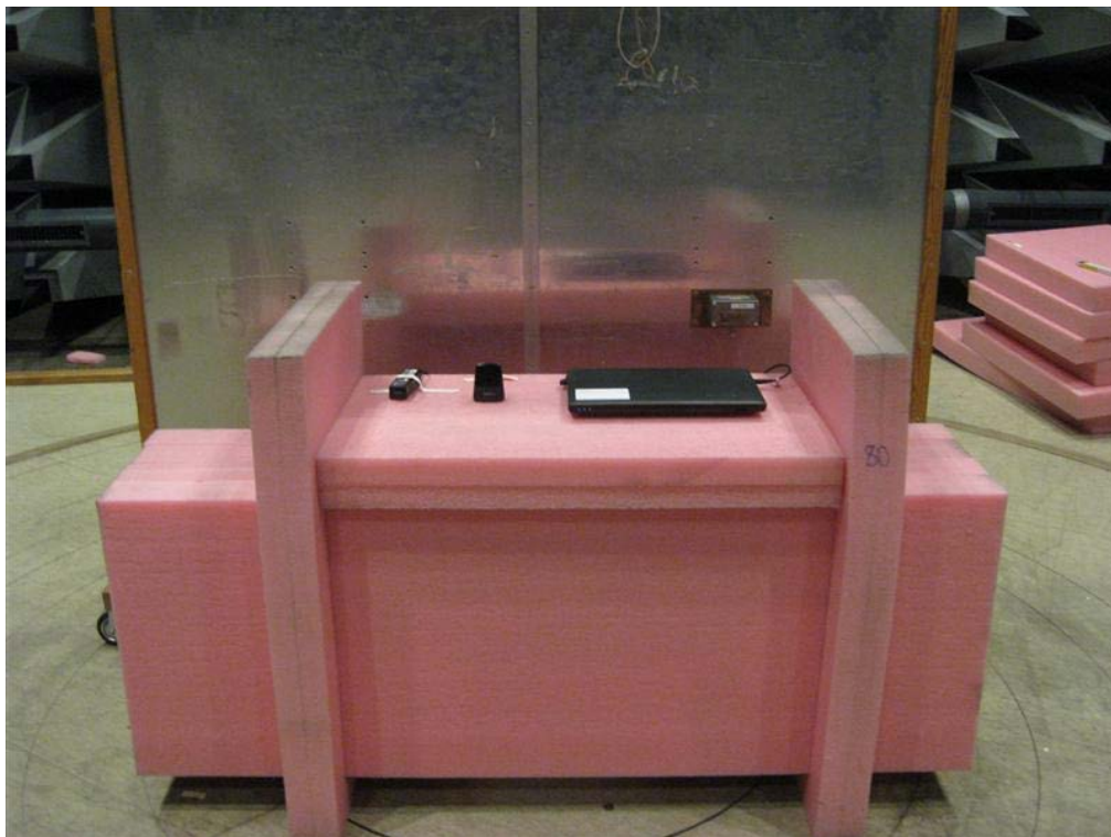
Photo 4.3.1 Test setup regarding measurement of radio frequency voltage on mains.
