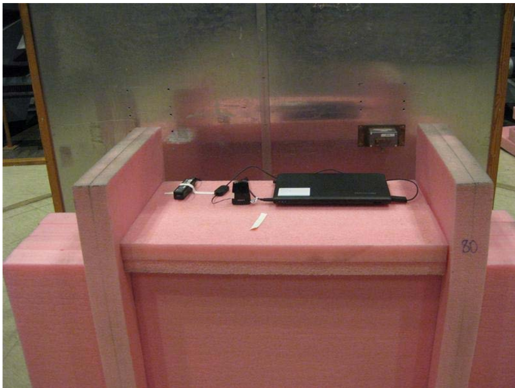
Photo 4.4.1 Test setup regarding measurement of radio frequency voltage on mains.
