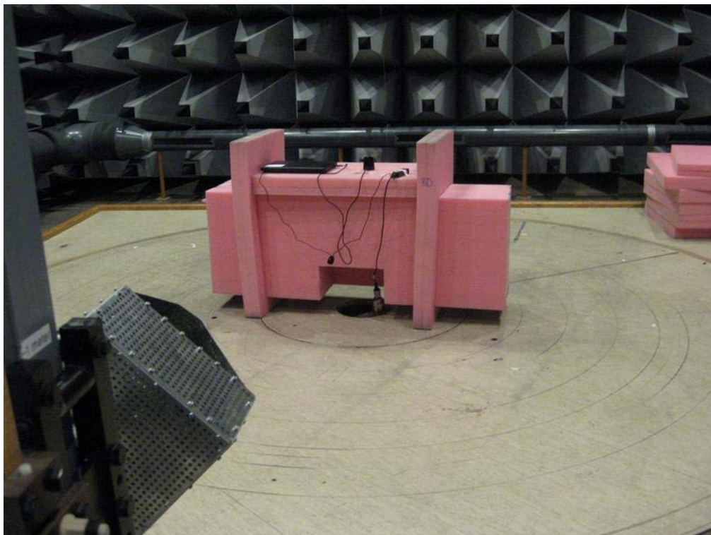
Photo 4.9.1 Test setup regarding measurement of radiated emission above 1 GHz.
