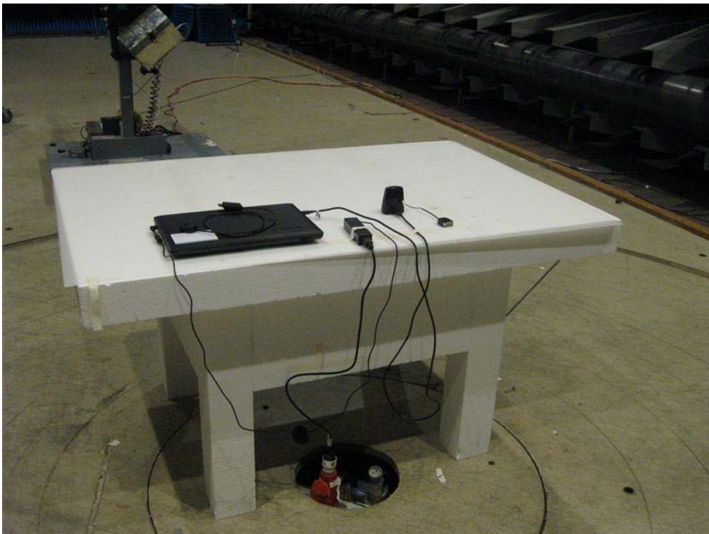
Photo 4.10.2 Test setup regarding measurement of radiated emission above 1 GHz.
