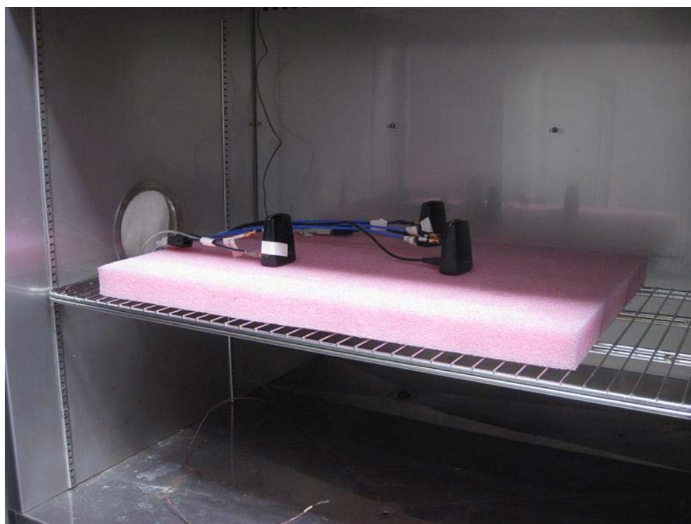
Photo 4.15.2 Test setup regarding measurement of 20 dB bandwidth.
